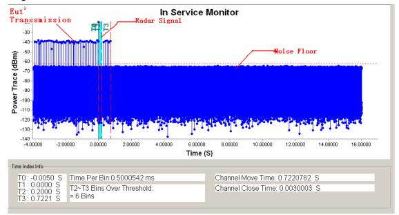
Note: T1 denotes the start of Channel Move Time upon the end of the last Radar burst.
