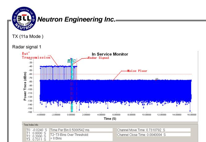
T1 denotes the start of Channel Move Time upon the end of the last Radar burst. Note:
