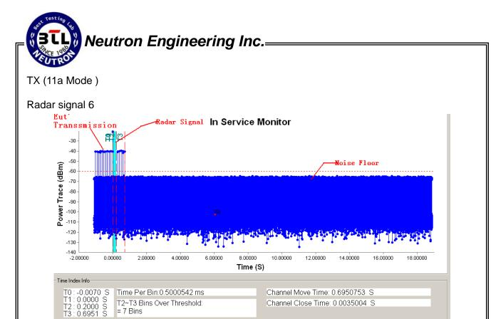
Note: T1 denotes the start of Channel Move Time upon the end of the last Radar burst.
