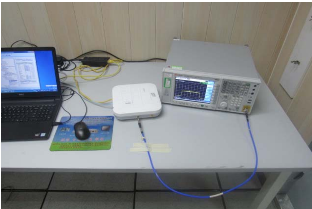
Picture 5 Conducted Test Setup
