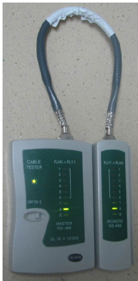
Figure 5-39 Testing the conduction and connections of wires
