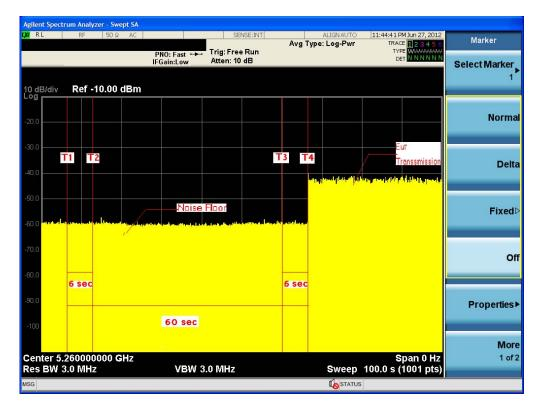
**Note:** T1 denotes the end of power-up time period is 7 second. T4 denotes the end of Channel Availability Check time is 67 second. Channel Availability Check time is equal to (T4 – T1) 60 seconds.
