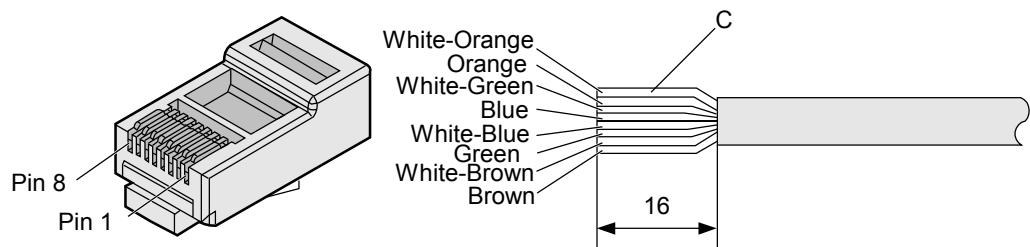
**Table 5-6** Connections between wires and pins (using a straight-through cable as an example)
