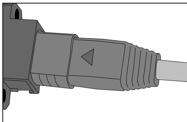
**Step 4** To disassemble an MPO fiber connector, hold the shell labeled "PULL" and remove the male connector, as shown in [Figure 5-71](#).
