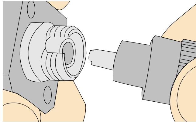
**Step 3** Feed the male connector into the female connector, as shown in [Figure 5-59](#).
