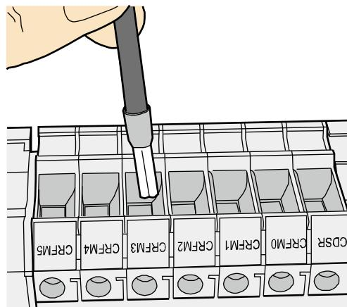
**Step 2** Insert the terminal into the jack vertically, and fasten the terminal by turning the matching screw in the clockwise direction, as shown in [Figure 5-49](#).
