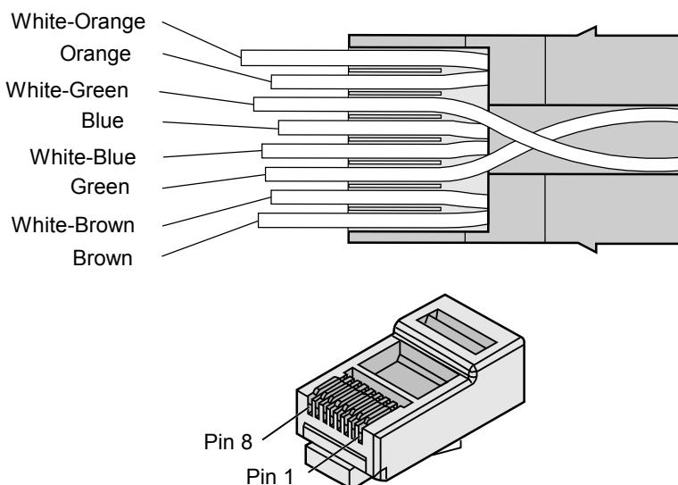
**Table 5-5** Connections between wires and pins (using a straight-through cable as an example)
