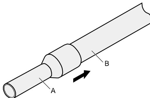
**Step 3** Crimp the joint parts of the cord end terminal and the conductor, as shown in [Figure 5-14](#).
