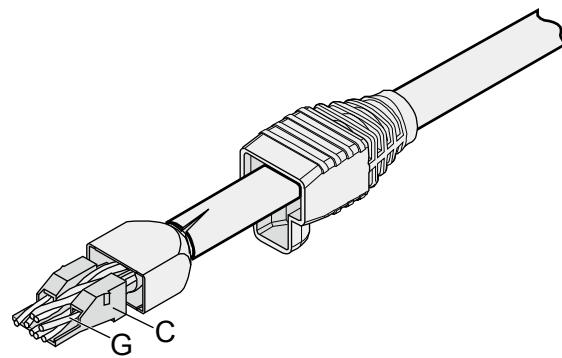
**Figure 5-21** Cable locations in a wire holder
