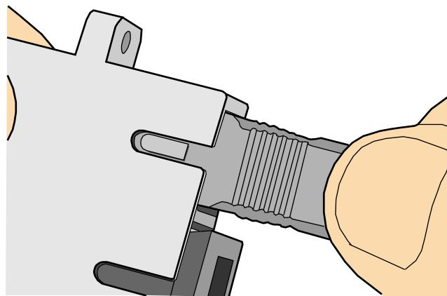
**Step 4** Before you disassemble an SC fiber connector, unlock the male connector by removing it slightly, as shown in [Figure 5-68](#).
