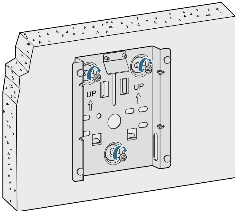
4. Align the mounting holes at the rear of the AP with the mounting screws on the mounting bracket and hang the AP on the bracket. Press the AP downwards to secure the AP on the wall.
