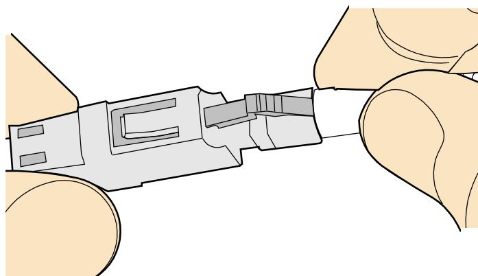
**Step 4** A clicking sound indicates that the male connector is locked, as shown in **Figure 5-64**.
