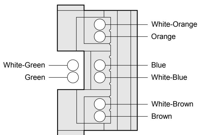
**Step 6** Align the four pairs of cables in the holder, as shown in [Figure 5-22](#). The connections between the wires and the pins are shown in [Figure 5-23](#) and listed in [Table 5-5](#).
