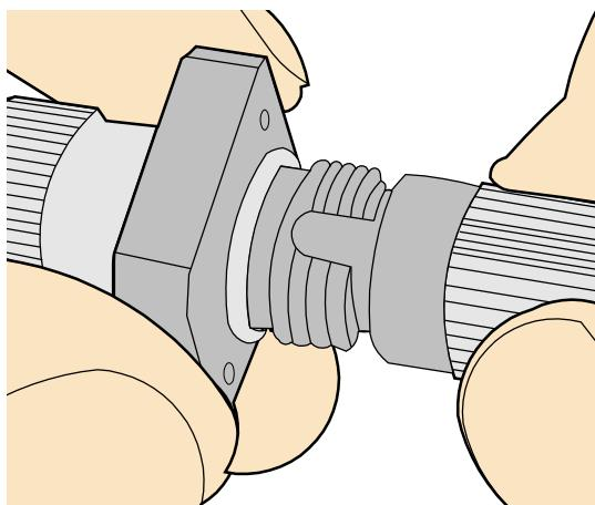
**Step 4** Fasten the locking nut in the clockwise direction and ensure that the connector is securely installed, as shown in [Figure 5-60](#).
