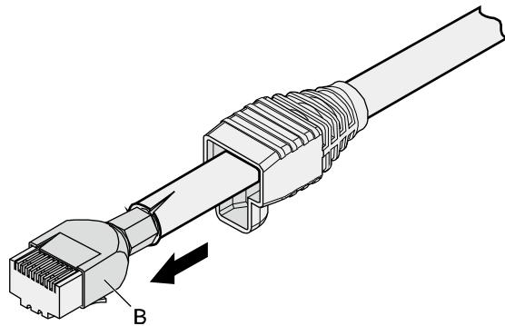
**Step 10** Push the jacket towards the metal shell until the metal shell is covered. This completes the assembly of one end of the cable, as shown in **Figure 5-27**.
