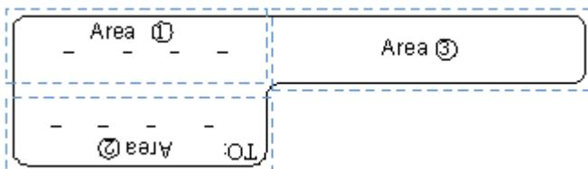
Seen from the cabling end of the equipment, the text part of the label is on the right side of the cable. The side with "TO:" that is facing outside carries the location information of the opposite end; and the other side carries the location information of the local end.
