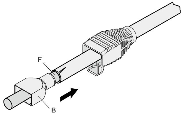
**Step 4** Fit the metal shell onto the twisted-pair cable until the shield layer is covered completely. Along the edge of the metal shell, cut off the aluminum foil shield layer and ensure that there is no surplus copper wire. The exposed twisted-pair cable is about 20 mm (0.79 in.) long, as shown in [Figure 5-19](#).
