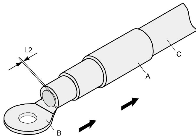
**Step 3** Put the OT terminal onto the exposed conductor, and ensure that the OT terminal is in good contact with the insulation of the power cable, as shown in [Figure 5-3](#).
