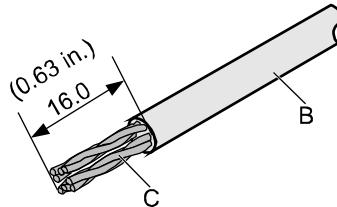
**Step 2** Align the four pairs of wires and cut the ends neatly, as shown in [Figure 5-30](#). The connections between the wires and the pins are listed in [Table 5-6](#).
