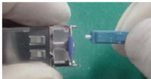
3. Cover unused optical connectors with protective caps, as shown in **Figure 5-99**, and then lay out fibers on the fiber rack or coil them in a fiber management tray to prevent fibers from being squeezed.
