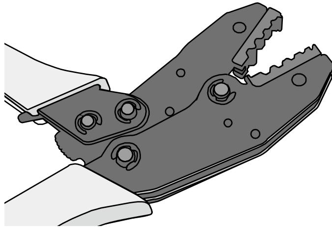
**Step 3** Remove the mould from the COAX crimping tools, as shown in [Figure 5-74](#).
