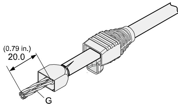
**Step 5** Based on the colors, lead the four pairs of twisted-pair wires through the wire holder, as shown in [Figure 5-20](#) and [Figure 5-21](#).
