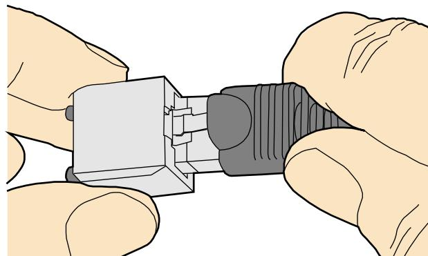
**Step 3** When you hear a click, the cable connector is completely inserted in the port. (The clip on the cable connector pops up to fix the connector in the port.) Pull the connector slightly and ensure that it is securely connected.
