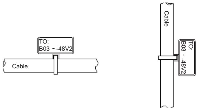
The identification card is on the top of the cable in horizontal cabling.
