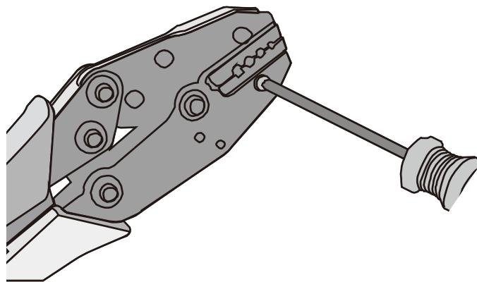
**Figure 5-78** shows the mold installed in the COAX crimping tool.
