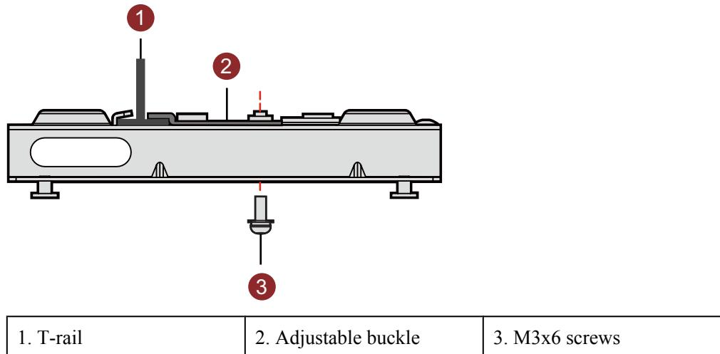
3. Align the mounting holes at the rear of the AP with the mounting screws on the sheet metal mounting bracket and secure the AP on the bracket.
