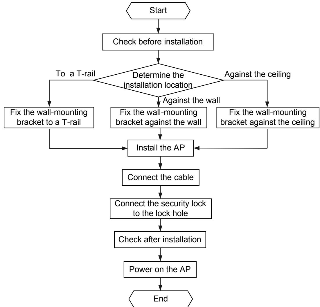
**Figure 2-3** Installation flowchart of the AP5030DN and AP5130DN
