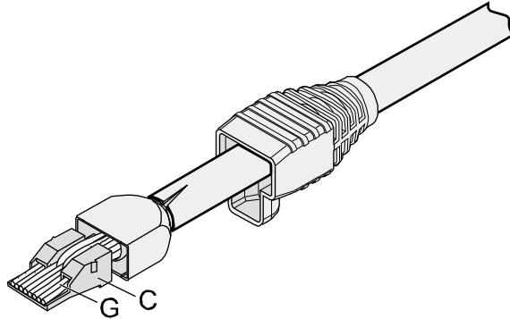
**Step 8** Put the connector body onto the wire holder and turn the metal shell by 90°, as shown in [Figure 5-25](#).
