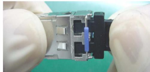
If no protective cap is available, use fibers to protect the optical module, as shown in **Figure 5-98**.
