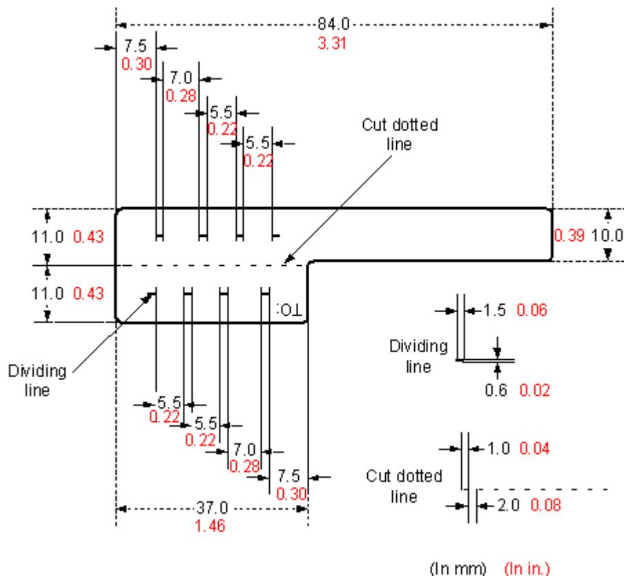
To specify more clearly the position of a cable, use the dividing lines on the label. For example, there is a dividing line between the cabinet number and the chassis number, and another one between the chassis number and the slot number. The dividing line is 1.5 mm x 0.6 mm (0.06 in. x 0.02 in.) with the color of Pantone 656c (light blue).
