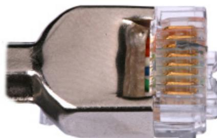
**Step 4** Check whether the contact strips and the plastic separators are well aligned and intact. If a separator is skew and cannot be fixed, replace it with a new RJ45 connector. [Figure 5-36](#) shows an unqualified piece.
