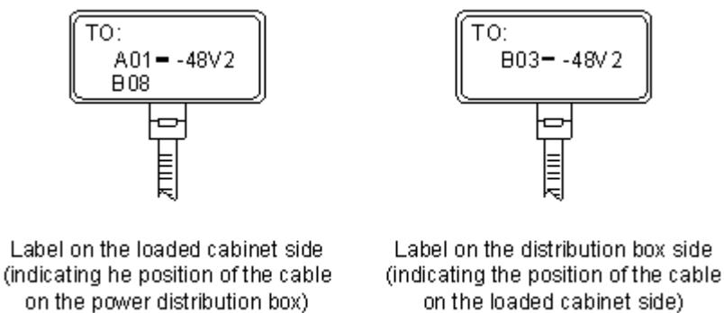
The meaning of the label in [Figure 5-93](#) is as follows:
