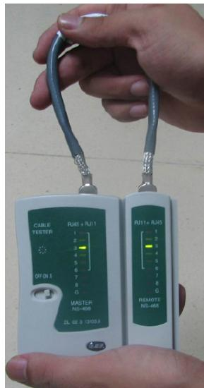
The procedure for testing a crossover cable is the same as that for testing a straight-through cable except for the sequence in which the indicators turn on. You need to refer to the wire connections of a crossover cable.
