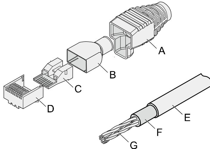
A. Jacket of connector      B. Metal shell of connector      C. Wire holder of connector      D. Plug of connector
