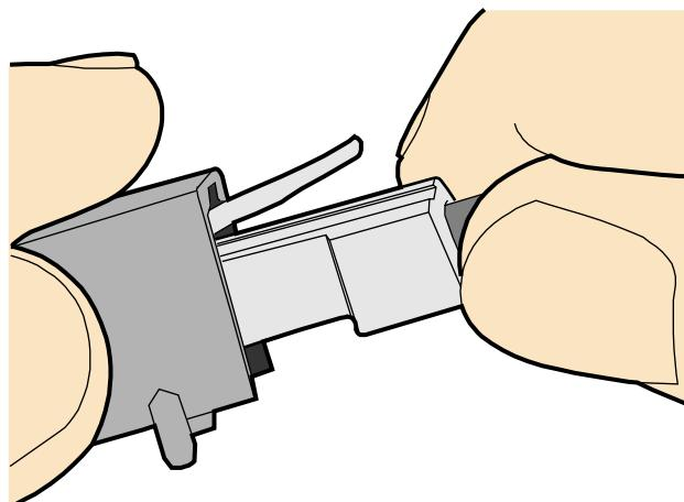
**Step 3** A crisp click indicates that the connector is locked by the locking key. Pull the connector slightly and ensure that it is securely connected. **Figure 5-56** shows an installed Ethernet connector.
