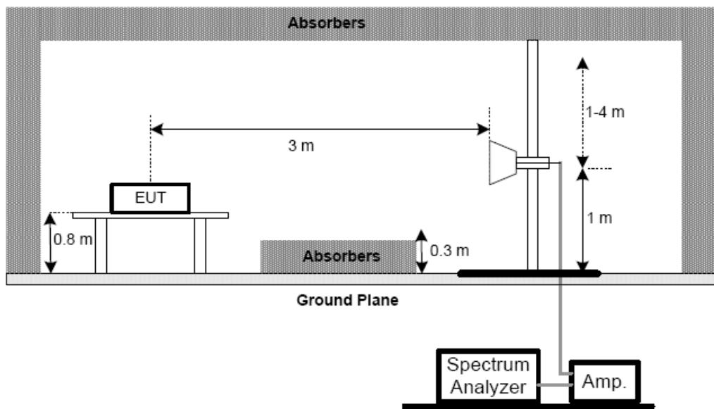
(C) For radiated emissions below 30MHz
