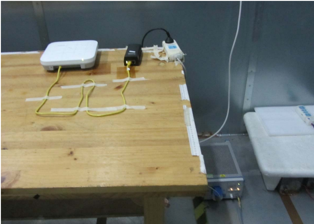
Picture 3 Conducted Emission Test Setup
