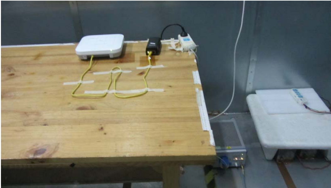
Picture 3 Conducted Emission Test Setup
