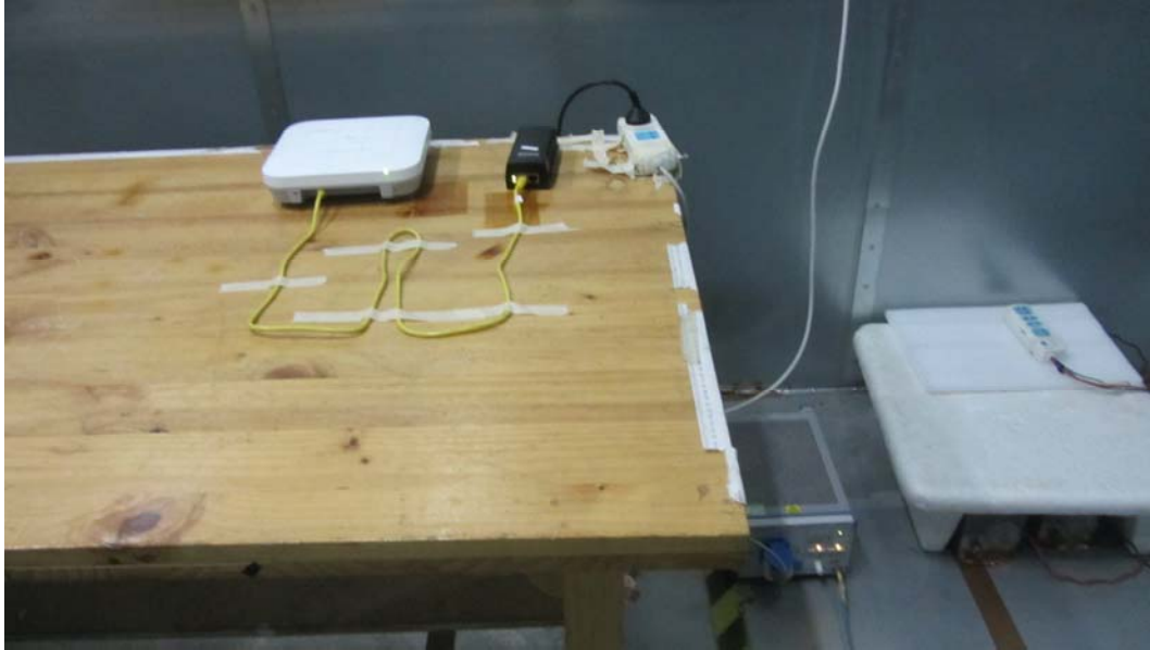
FCC Part15E Conducted Emission Test Setup
