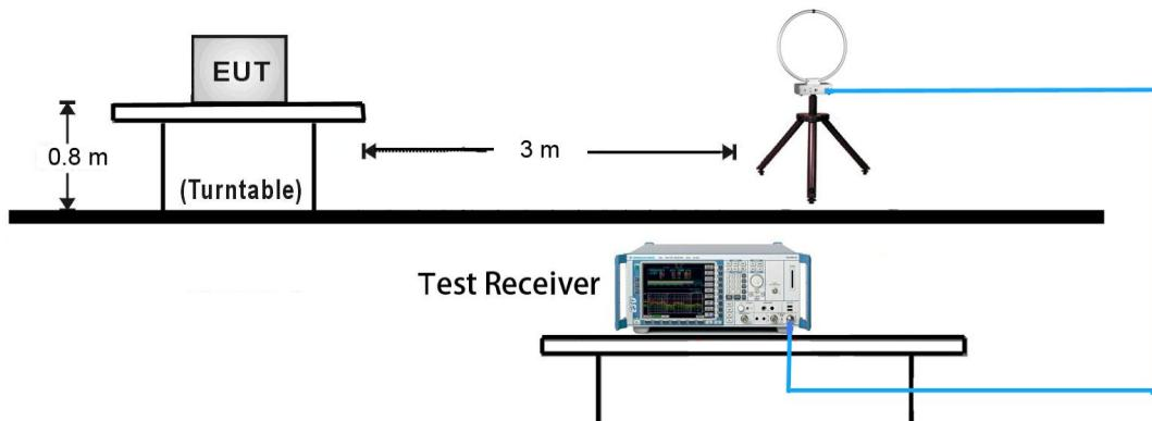
30MHz ~ 1GHz Test Setup:
