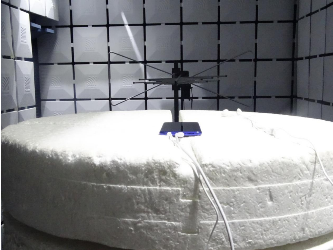
Radiated Spurious Emission (below 3GHz)
