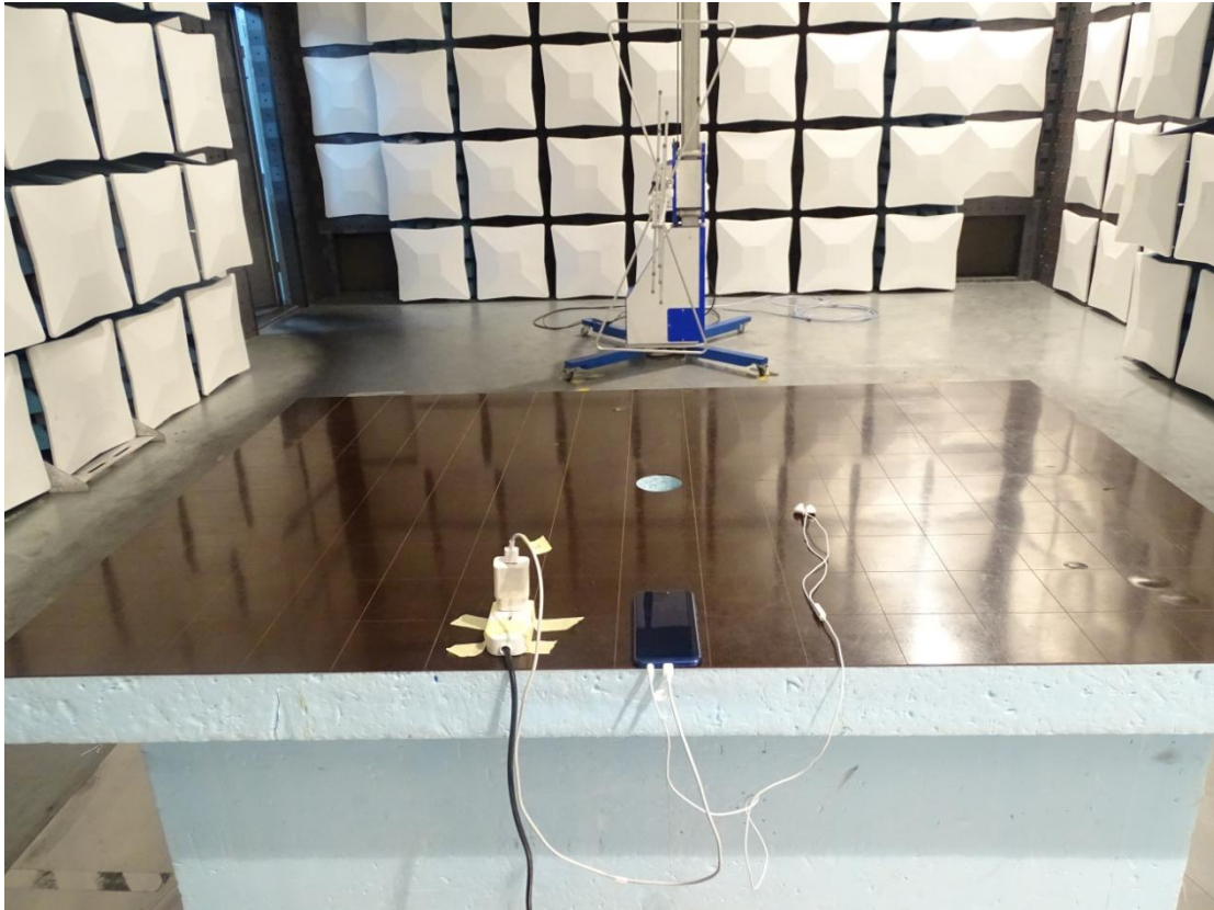
Radiated Spurious Emission (below 1GHz)
