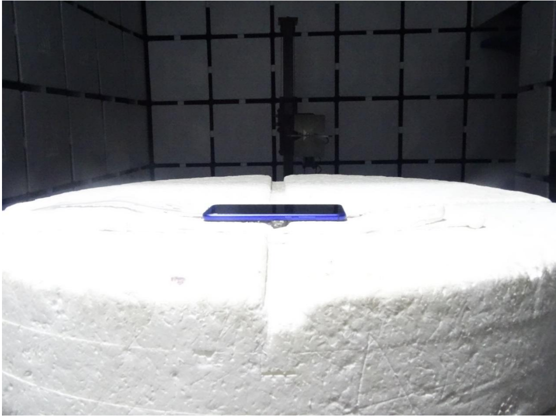
Radiated Spurious Emission (3GHz to18GHz)
