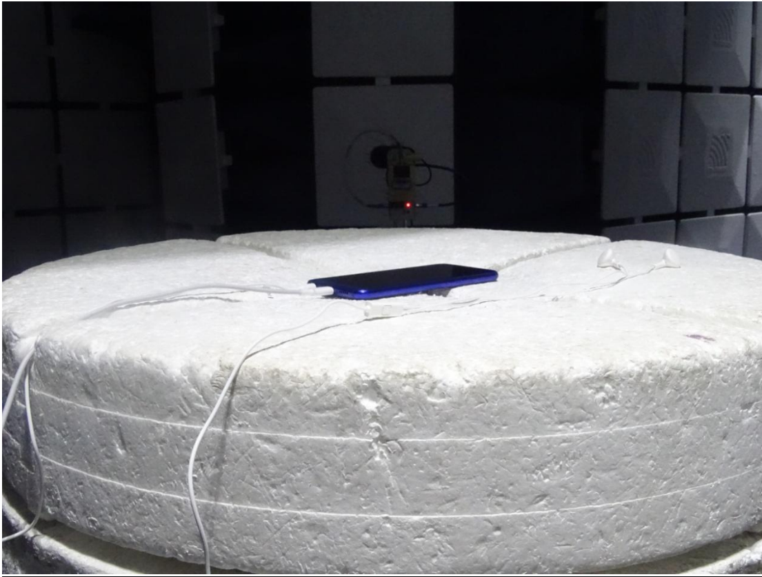
Radiated Spurious Emission (18GHz to26.5GHz)
