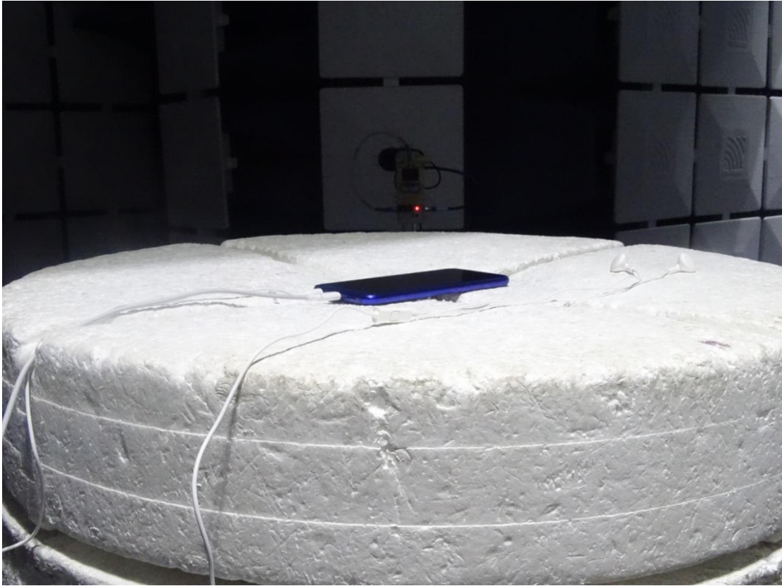
Radiated Spurious Emission (18GHz to26.5GHz)
