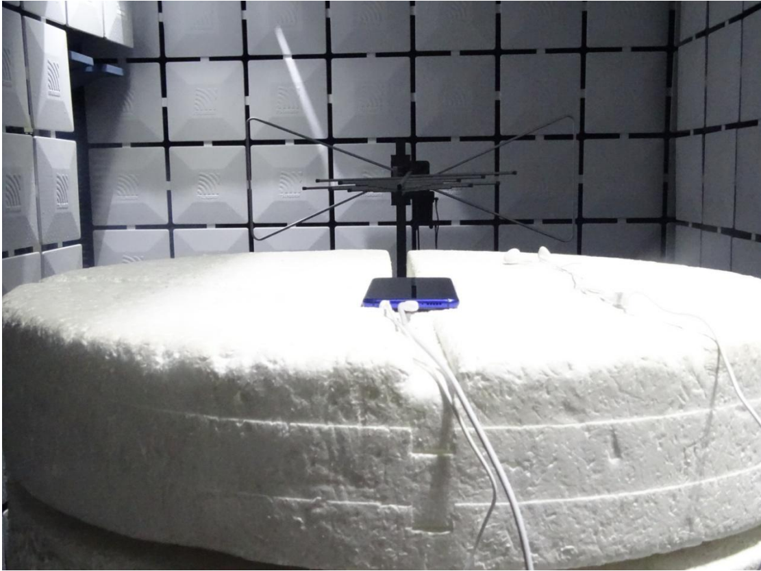
Radiated Spurious Emission (30MHz-3GHz)
