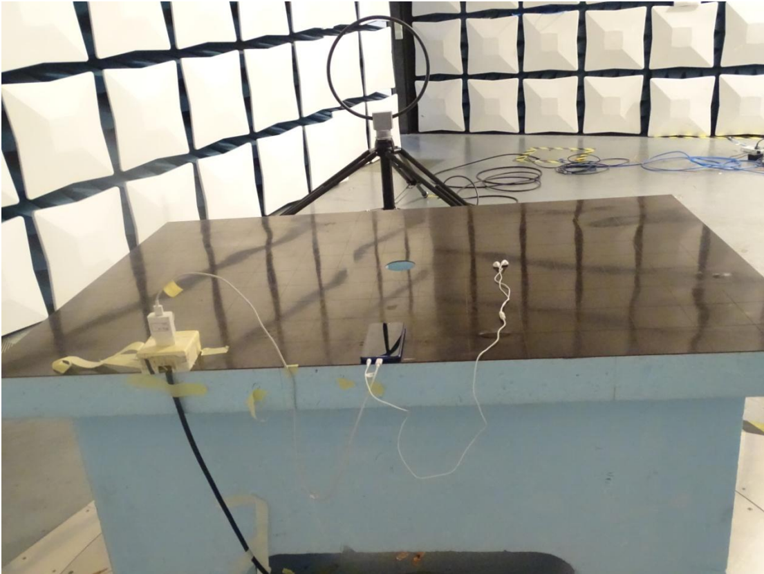
Radiated Spurious Emission (9K-30MHz)
