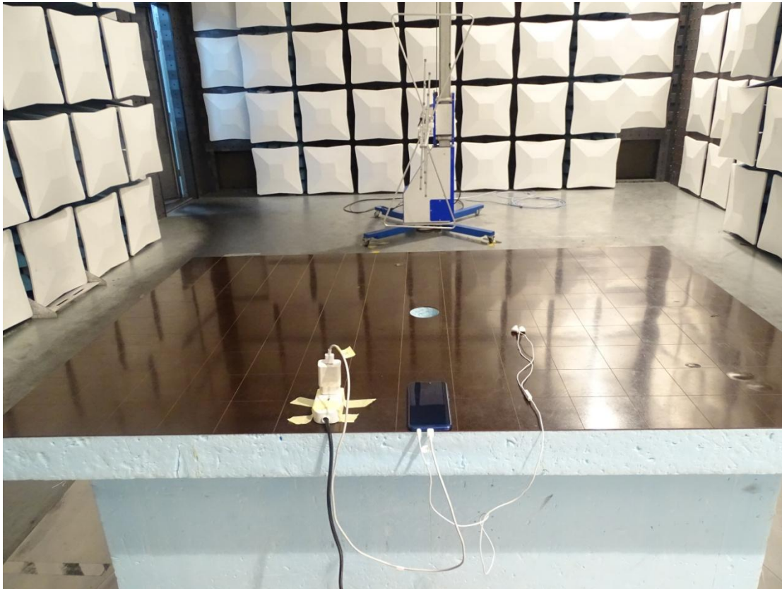
Radiated Spurious Emission (30MHz-1GHz)
