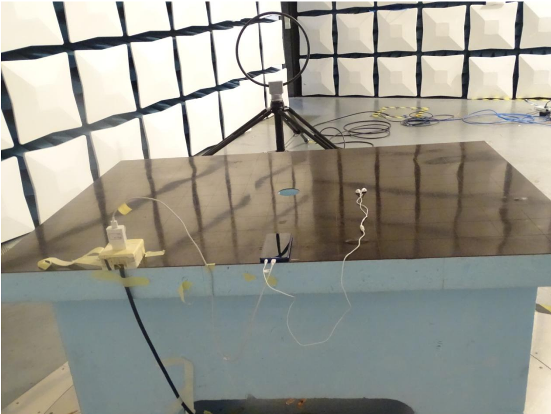
Radiated Spurious Emission (9K-30MHz)
