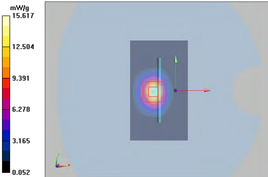
**Plot 8 System Performance Check at 2600 MHz Body TSL**
