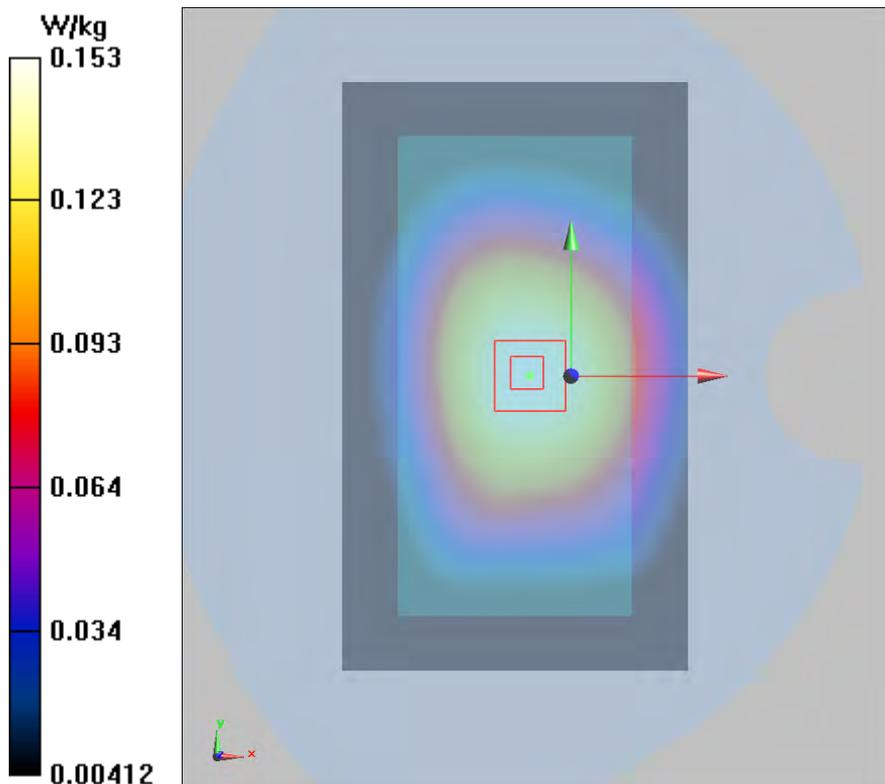
**Plot 14 GSM 1900 GPRS (4Txslots) Back Side Middle (Distance 10mm)**
