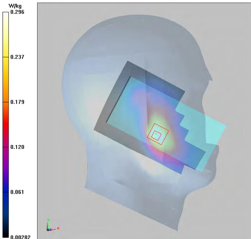
**Plot 13 GSM 1900 Back Side Middle (Distance 15mm)**
