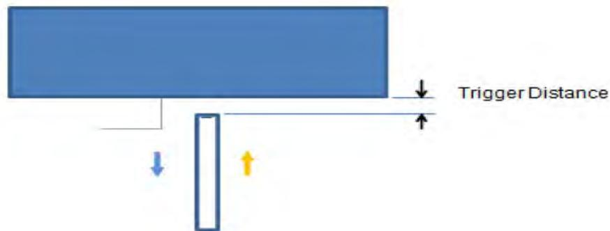
Picture: Proximity sensor triggering distances assessment (Bottomside)
