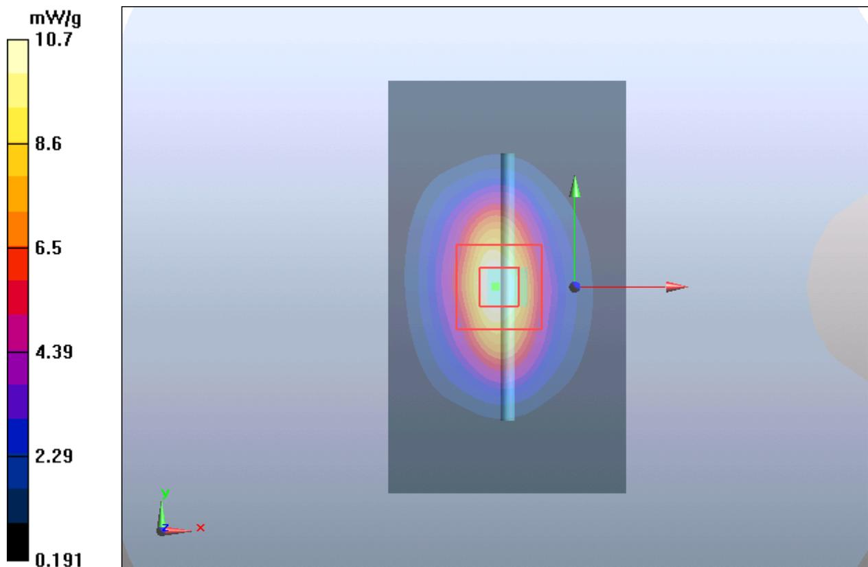
**Plot 4 System Performance Check at 1900 MHz Body TSL**
