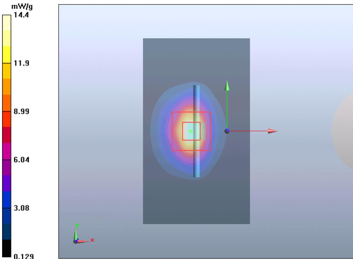
**Plot 7 System Performance Check at 2600 MHz Head TSL**
