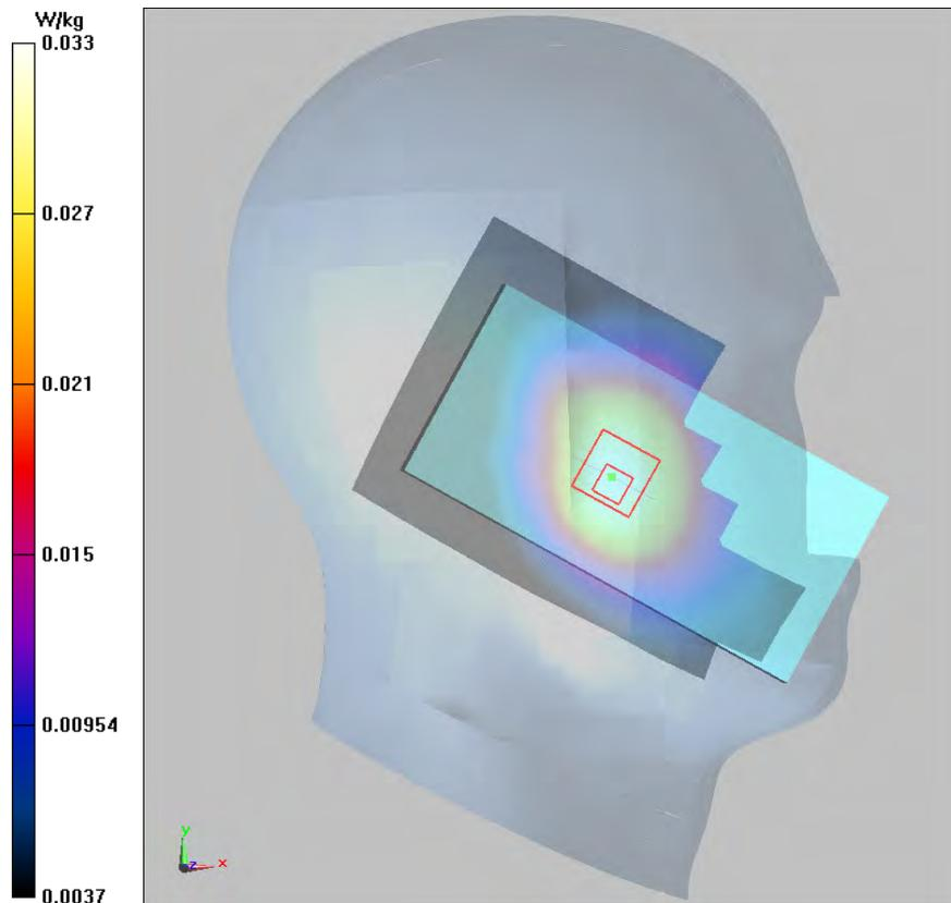
**Plot 10 GSM 850 Back Side Middle (Distance 15mm)**
