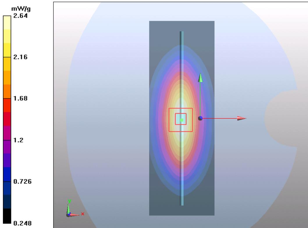
**Plot 2 System Performance Check at 835 MHz Body TSL**
