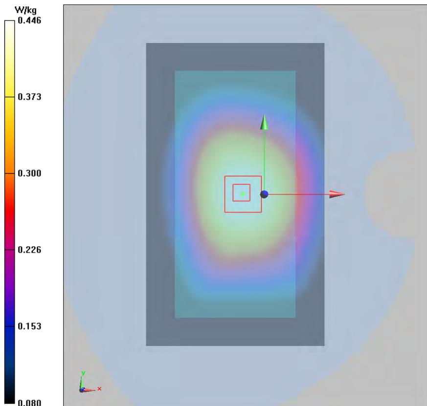
**Plot 11 GSM 850 GPRS (4Txslots) Right Edge Middle (Distance 10mm)**
