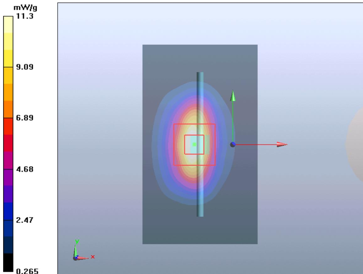
**Plot 5 System Performance Check at 2450 MHz Head TSL**
