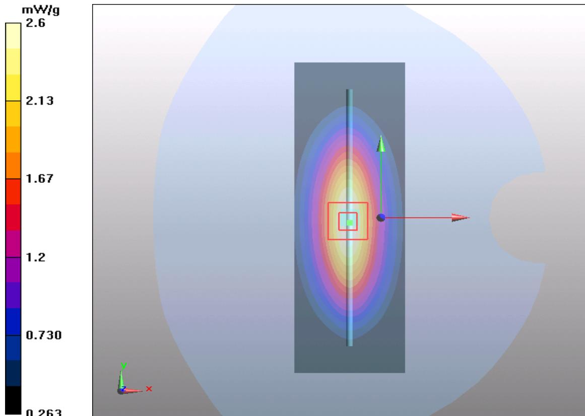
**Plot 3 System Performance Check at 1900 MHz Head TSL**
