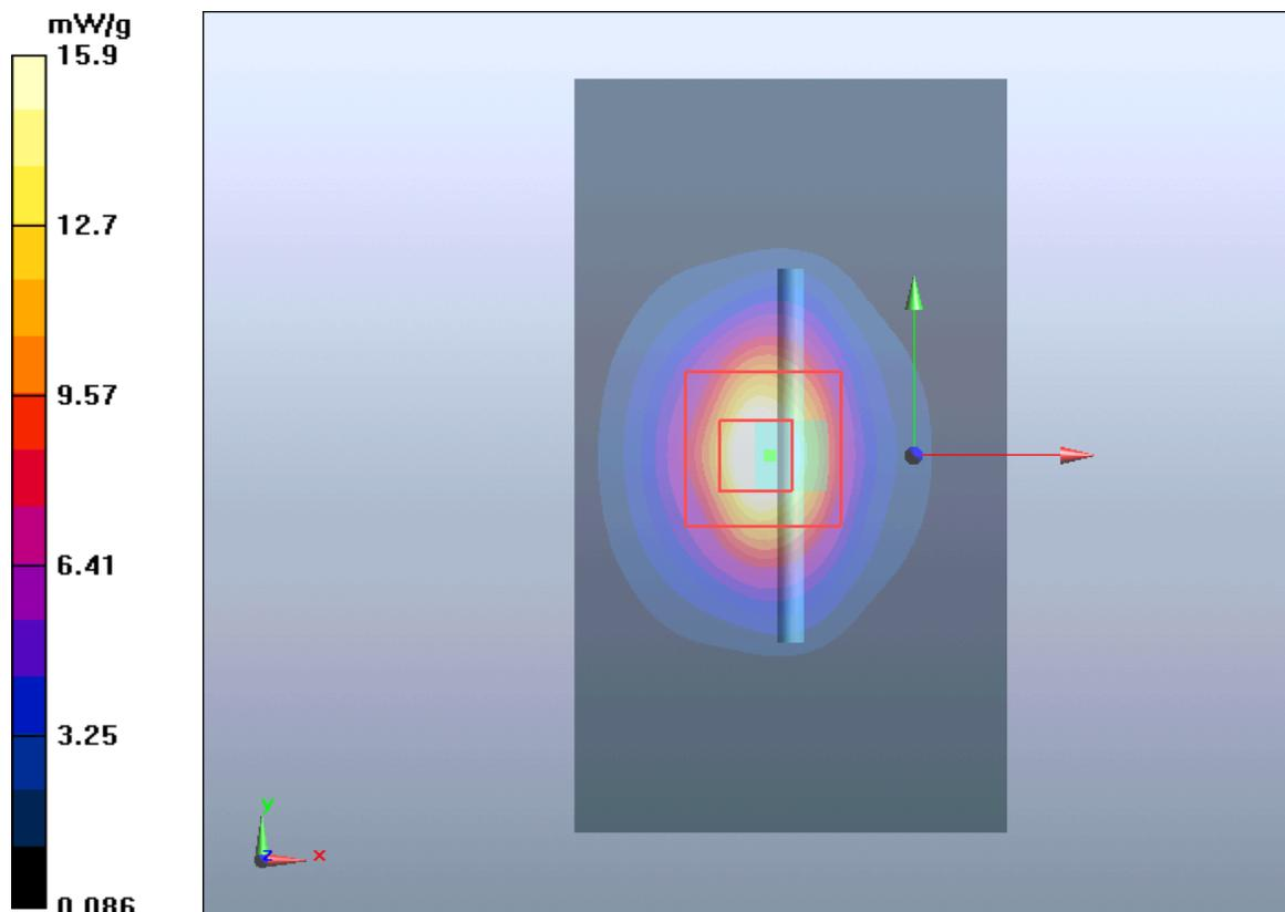
**Plot 6 System Performance Check at 2450 MHz Body TSL**
