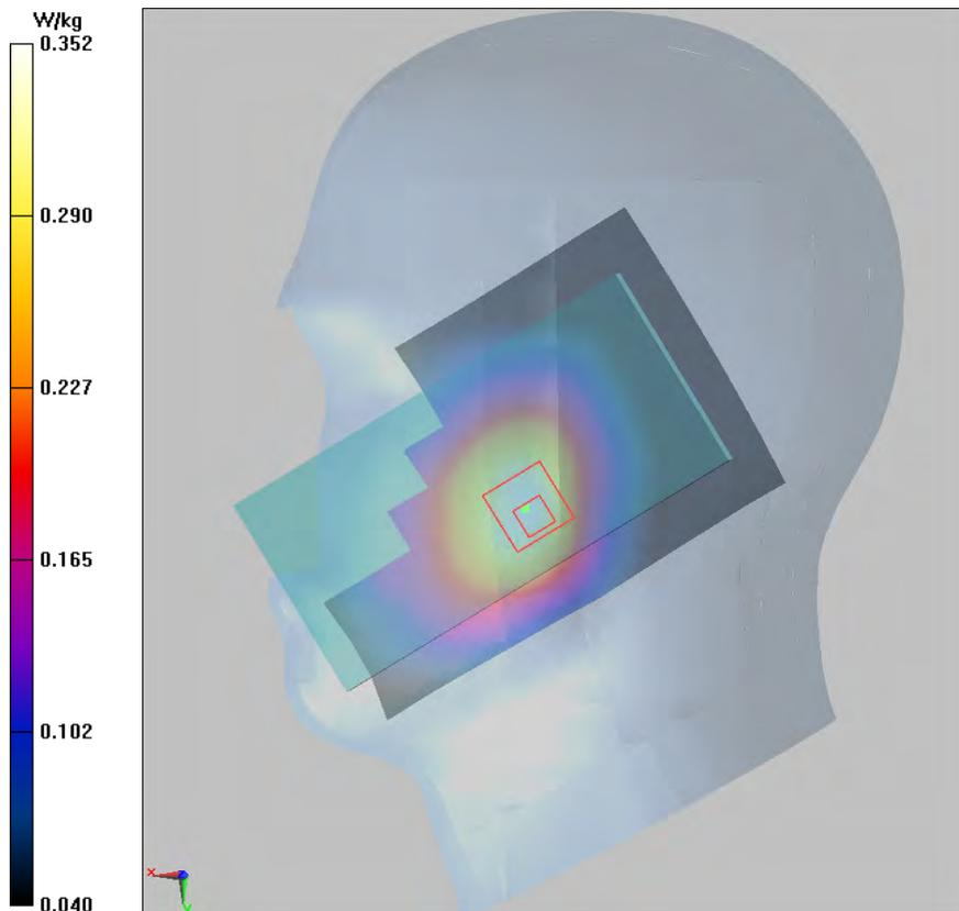
**Plot 16 UMTS Band V Front Side Middle (Distance 15mm)**
