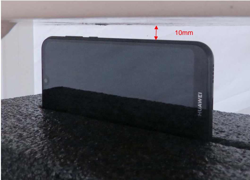
Picture 11: Right Side, the distance from handset to the bottom of the Phantom is 10mm
