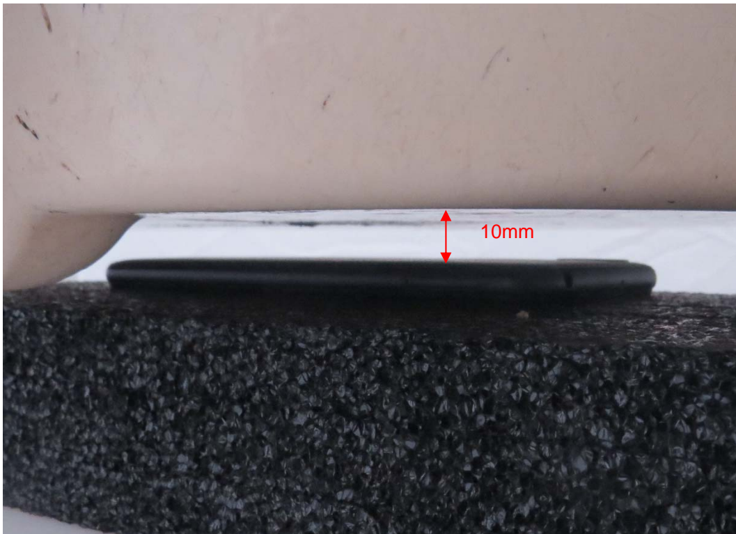
Picture 8: Back Side, the distance from handset to the bottom of the Phantom is 10mm
