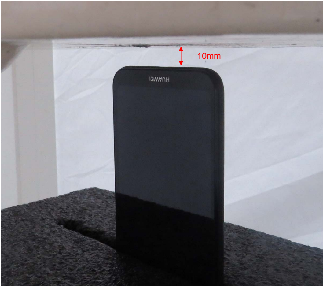
Picture 13: Bottom Edge, the distance from handset to the bottom of the Phantom is 10mm
