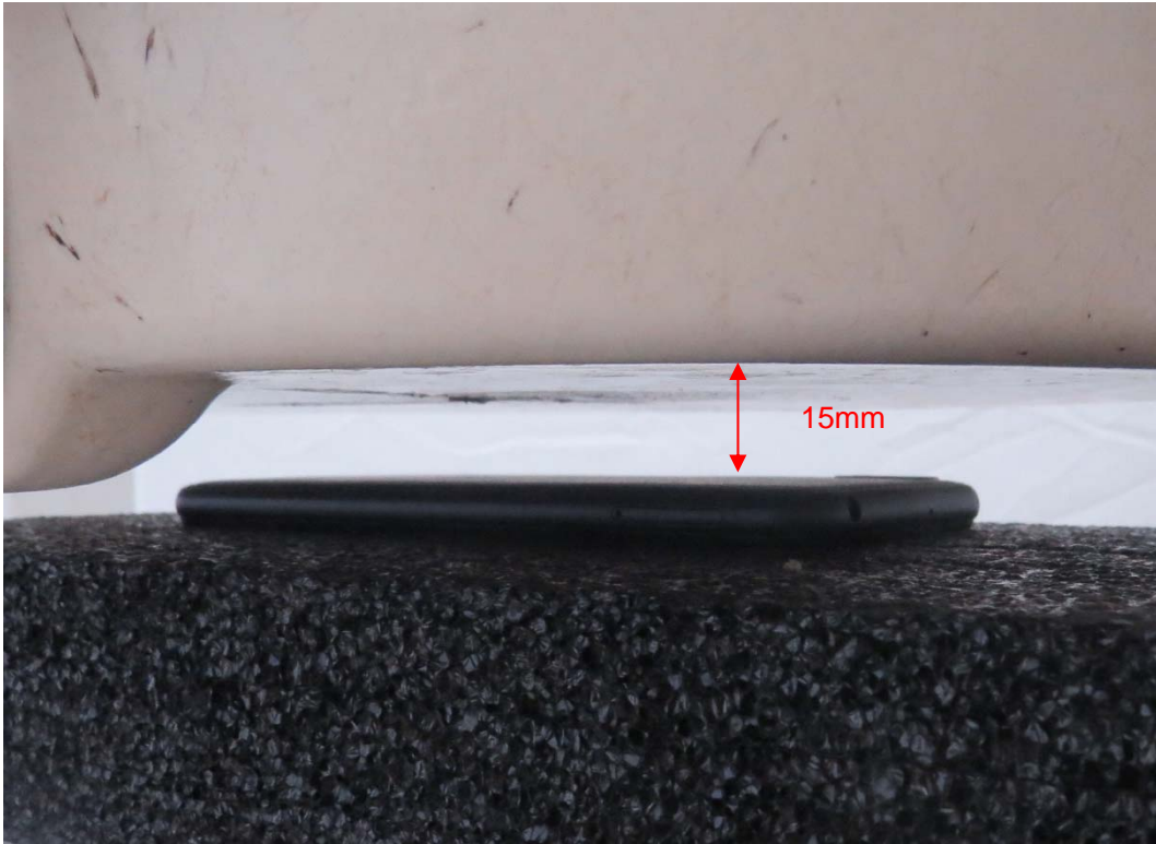
Picture 5: Back Side, the distance from handset to the bottom of the Phantom is 15mm
