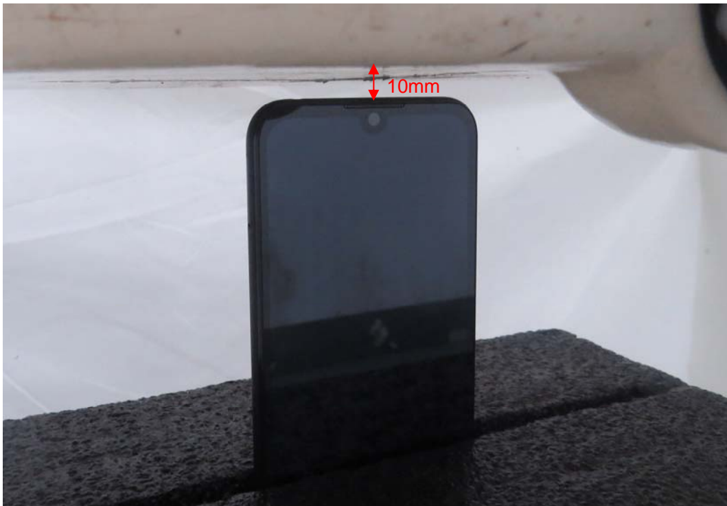
Picture 12: Top Edge, the distance from handset to the bottom of the Phantom is 10mm
