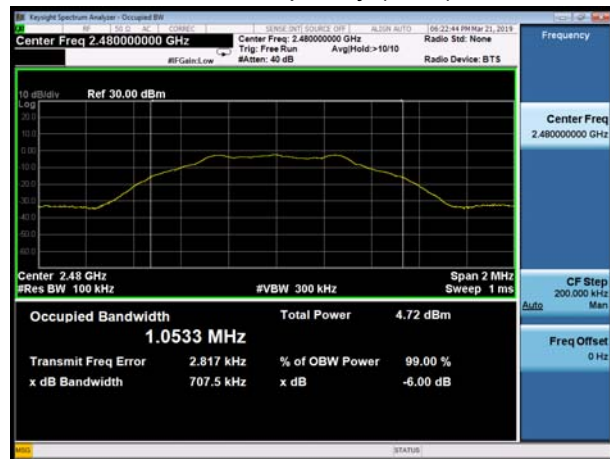
BLE Carrier frequency (MHz): 2480
