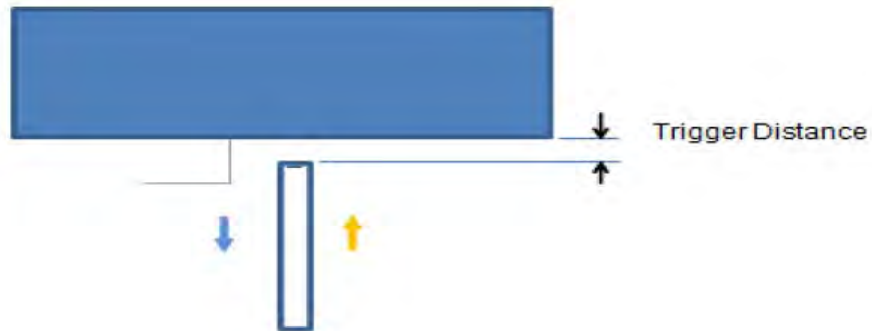
Picture: Proximity sensor triggering distances assessment (Bottomside)
