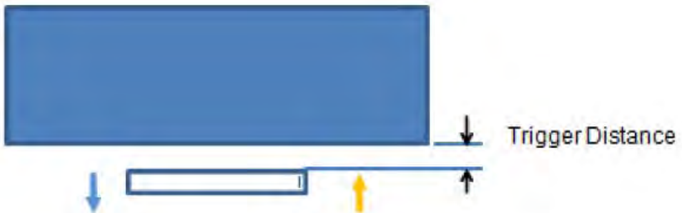
Picture: Proximity sensor triggering distances assessment (Front side)
