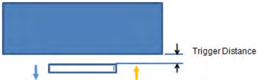
Picture: Proximity sensor triggering distances assessment (Back side)
