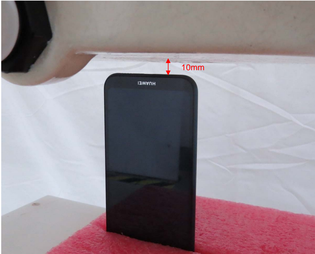
Picture 15: Bottom Edge, the distance from handset to the bottom of the Phantom is 10mm
