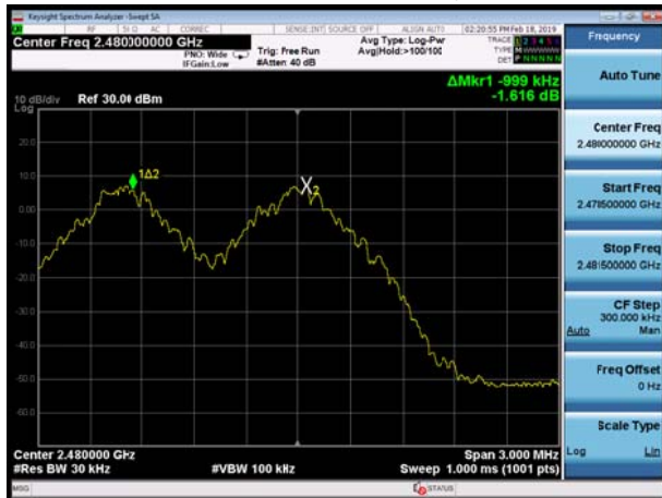
BT DH5 CH78, Carrier frequency (MHz): 2480
