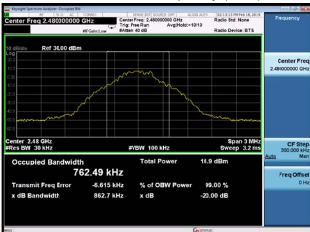
BT DH5 CH78, Carrier frequency (MHz): 2480
