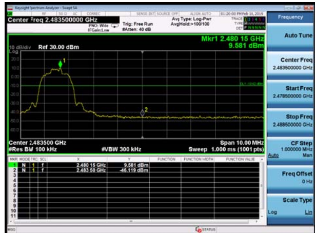
BT 3DH5 CH78, Carrier frequency (MHz): 2480
