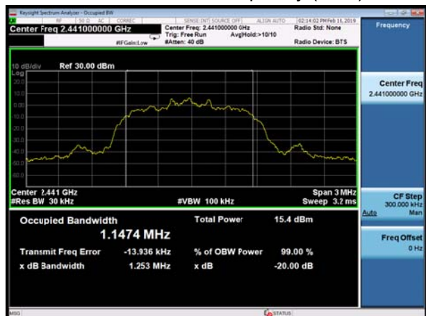
BT 2DH5 CH78, Carrier frequency (MHz): 2480
