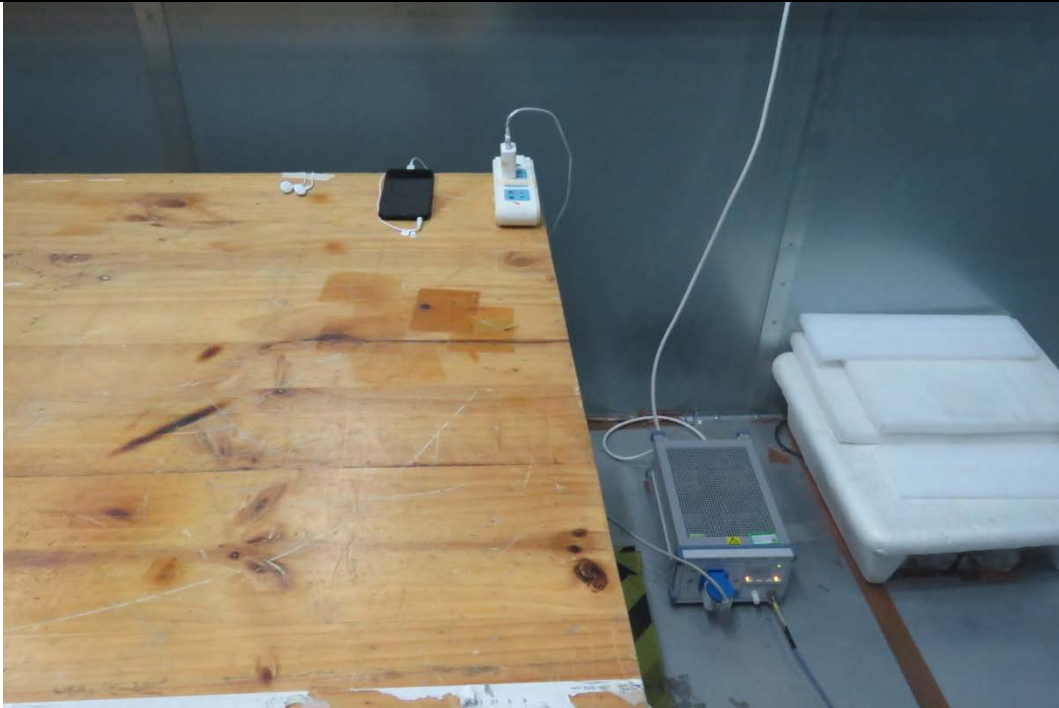
Picture 3 Conducted Emission Test Setup
