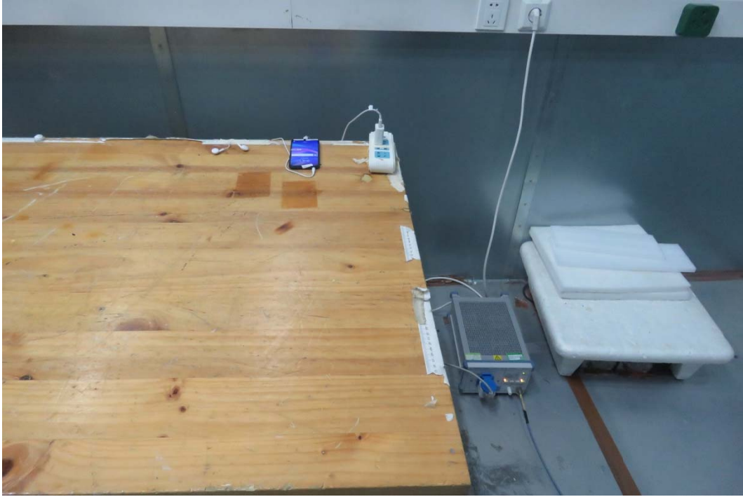
Picture 2 Conducted Emission Test Setup
