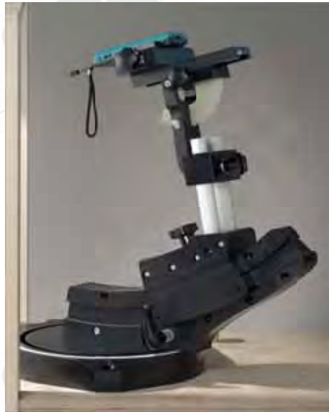
F-2. Device Holder for Transmitters
