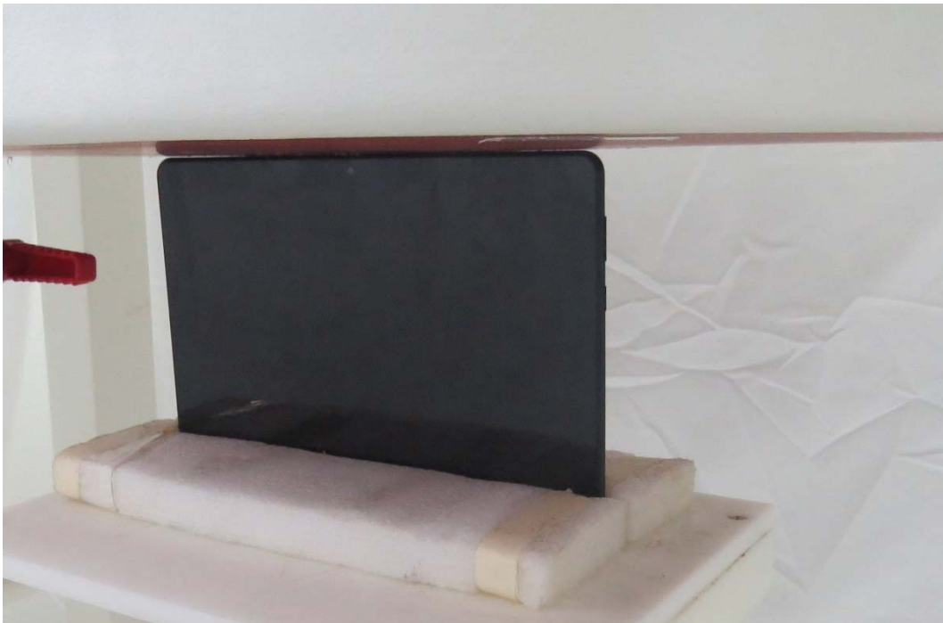
Picture 4: Top Side, the distance from handset to the bottom of the Phantom is 0mm
