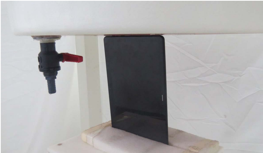
Picture 3: Right Side, the distance from handset to the bottom of the Phantom is 0mm
