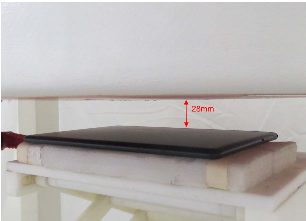
Picture 2: Back Side, the distance from handset to the bottom of the Phantom is 28mm
