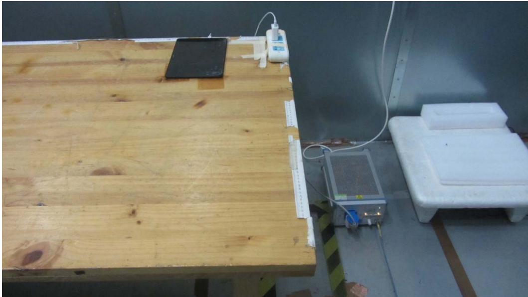
Picture 2 Conducted Emission Test Setup
