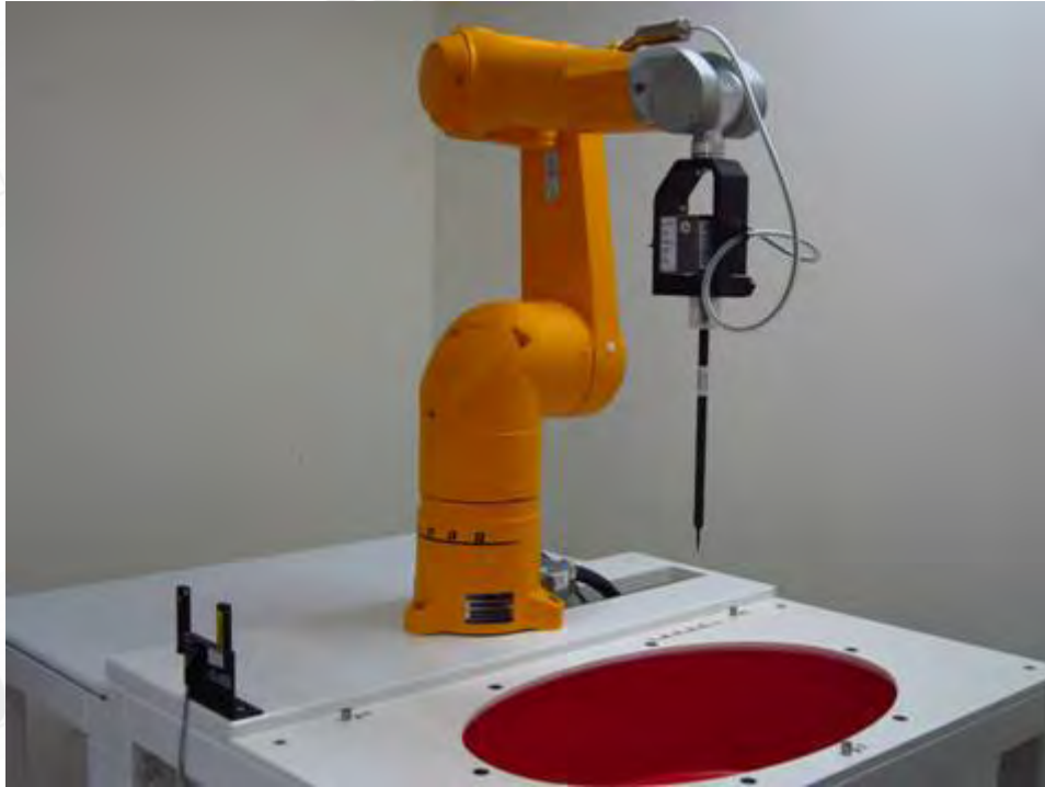
Fig.1 Photograph of the SAR measurement system
