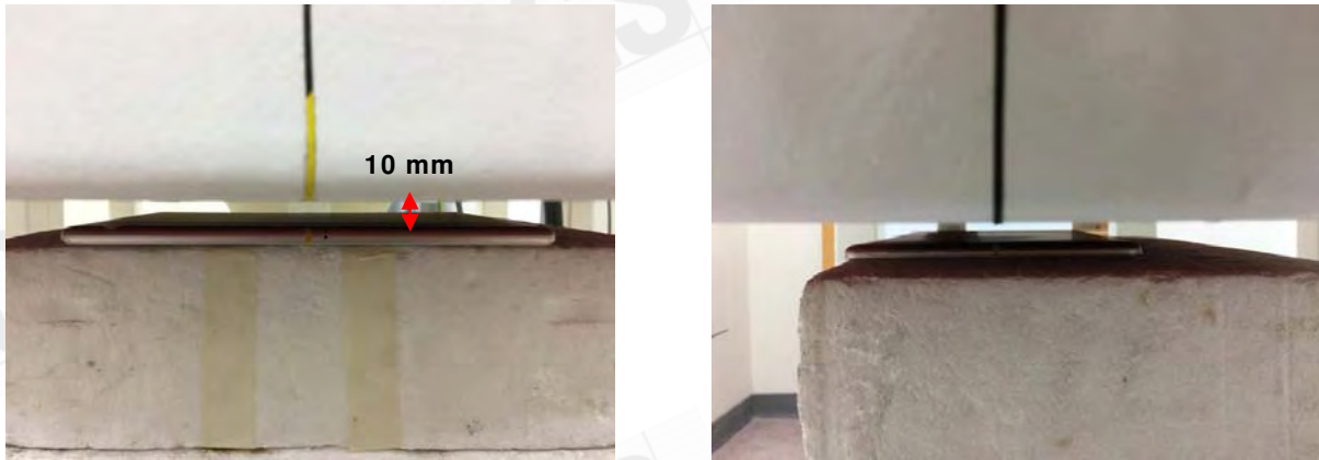
Fig.4 EUT Back side (10mm) to flat phantom
