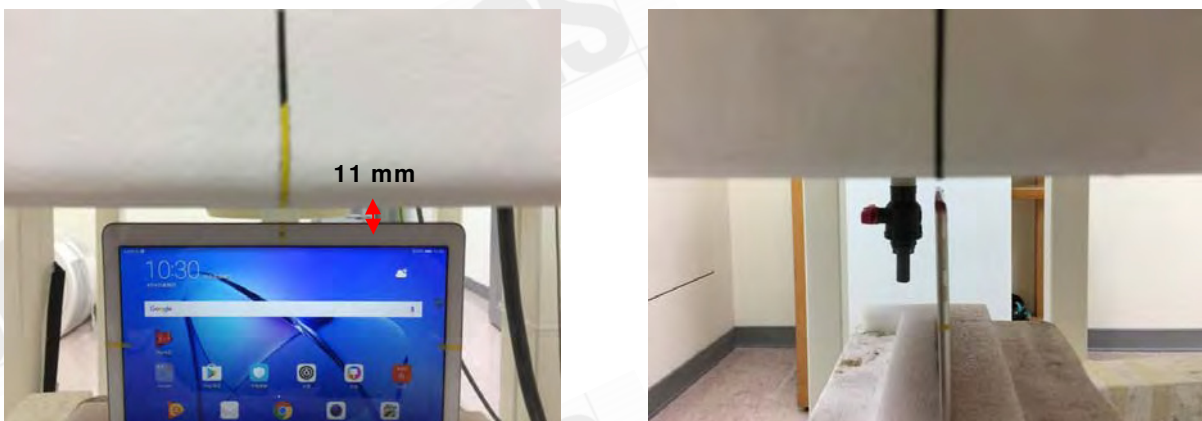
Fig.8 EUT Top side (11mm) to flat phantom
