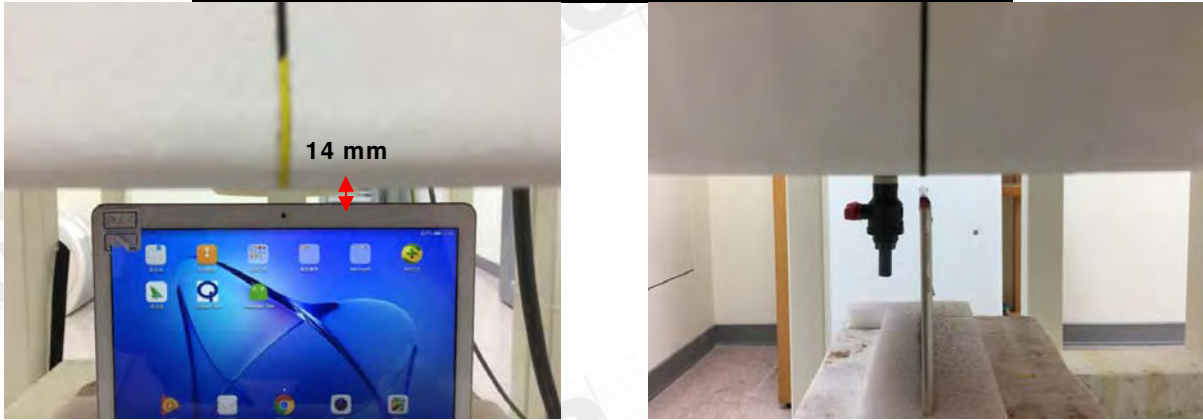
Fig.9 EUT Top side (14mm) to flat phantom
