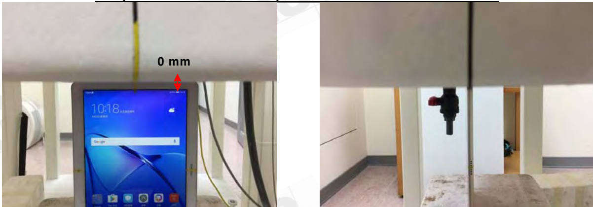
Fig.6 EUT Right side to flat phantom
