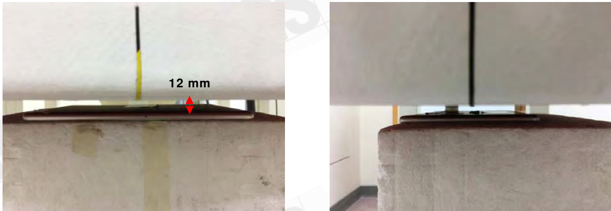
Fig.5 EUT Back side (12mm) to flat phantom
