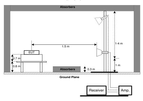
(C) For radiated emissions below 30MHz
