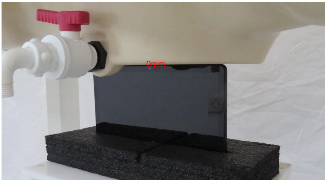
Picture 6: Top Edge, the distance from handset to the bottom of the Phantom is 0mm
