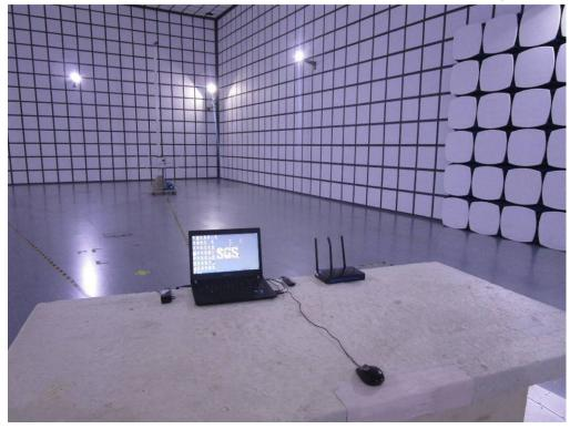
1.2 Conducted Disturbance at Mains Terminals(150kHz-30MHz) Test Setup
