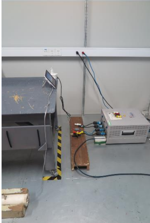
Conducted emissions of AC power port
