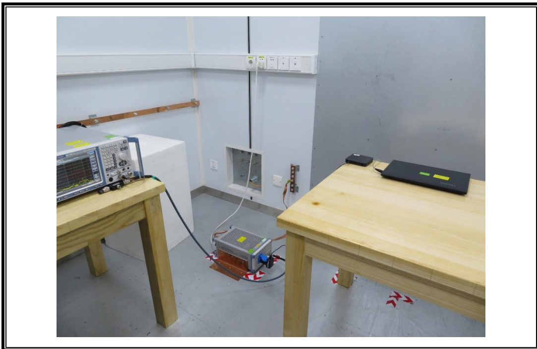
POWERLINE CONDUCTED EMISSIONS MEASUREMENT SETUP-1
