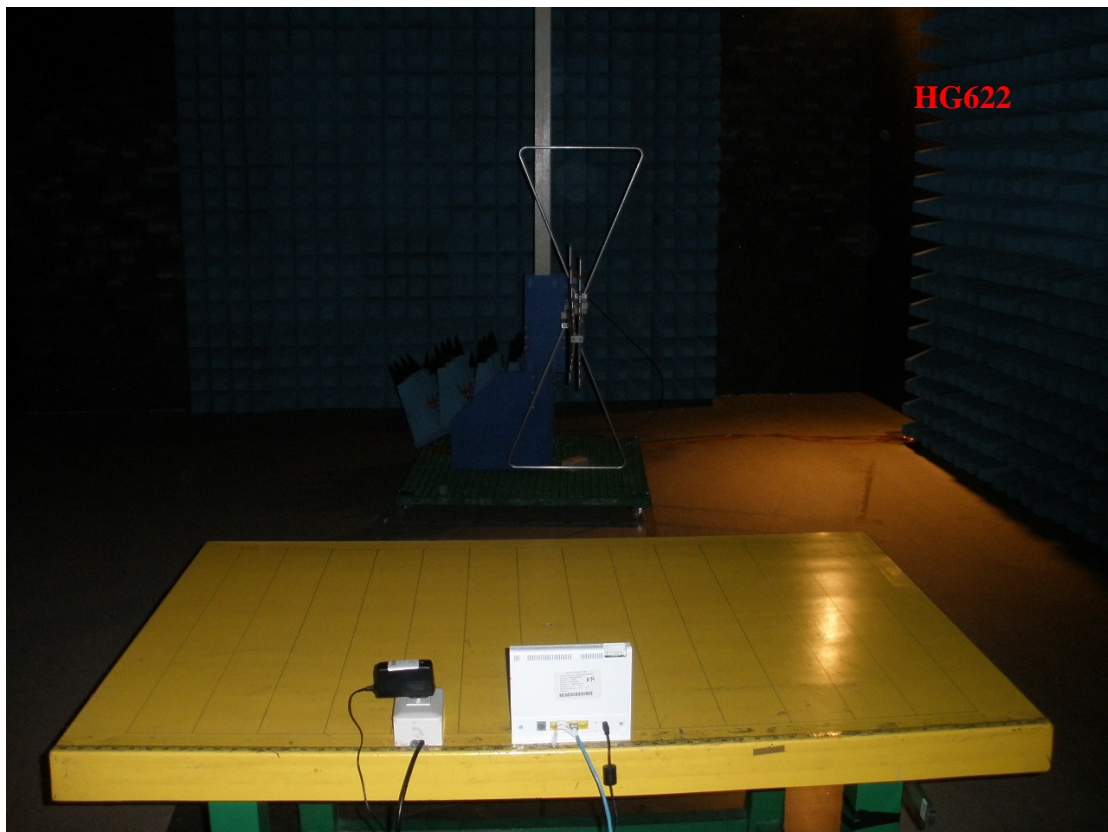
Photo 2: Radiated Emission Test set-up photo
