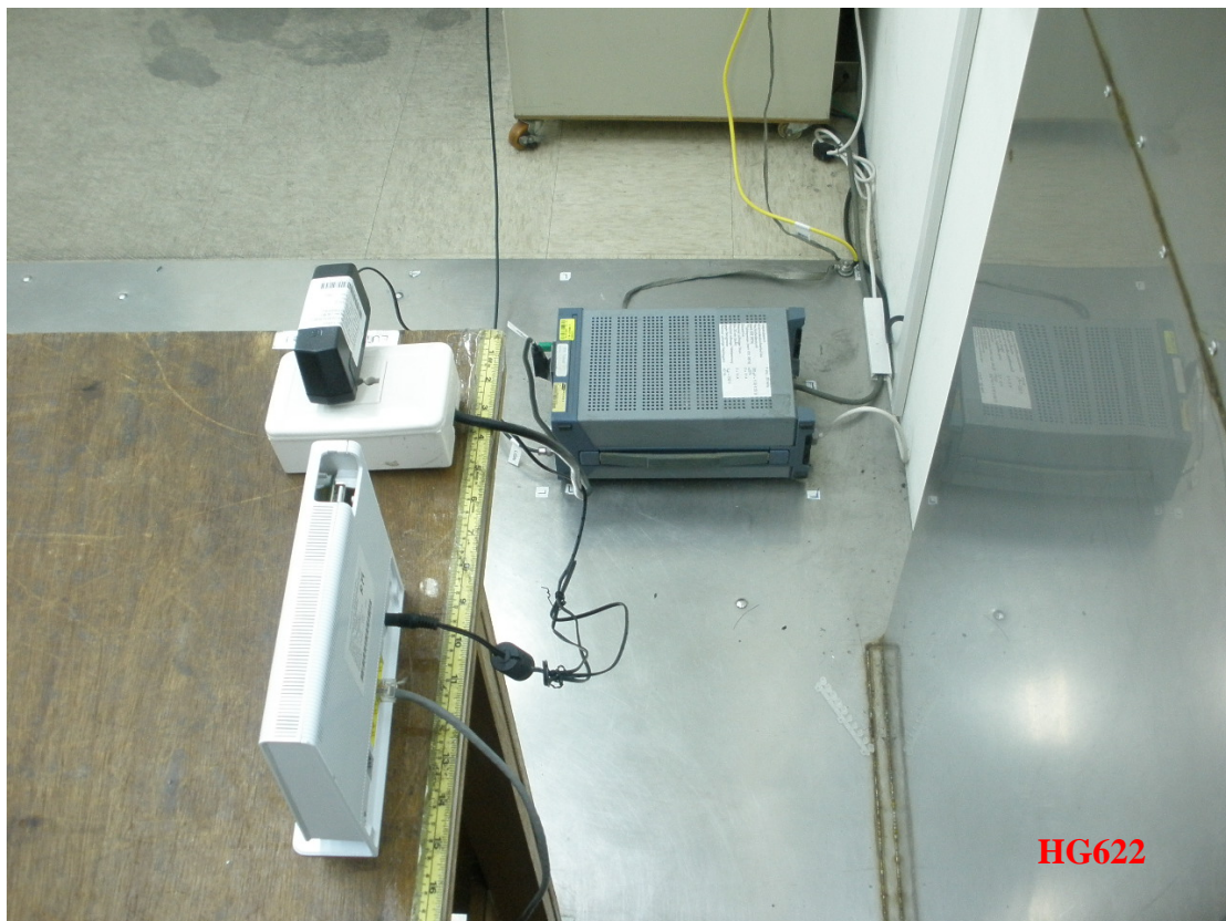
Photo 2: Conducted Emission Test Set-up photo
