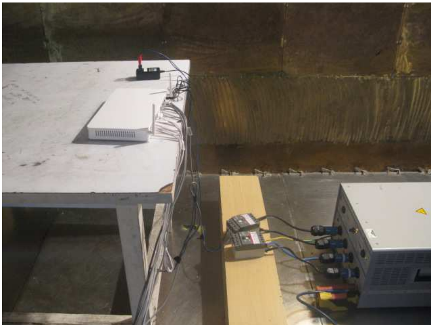
Conducted emissions of AC power port
