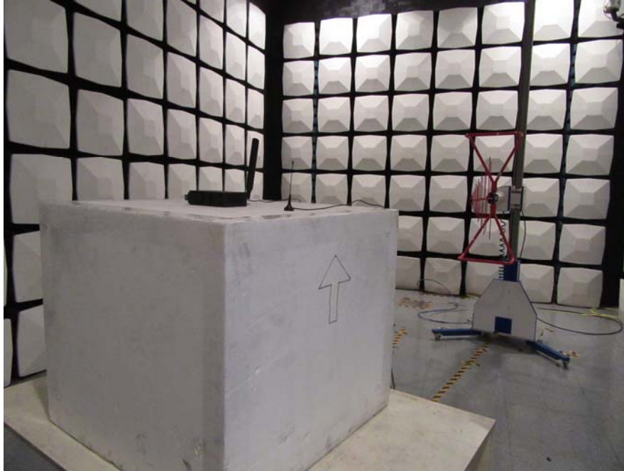
Radiated Emission View---Below 1GHz
