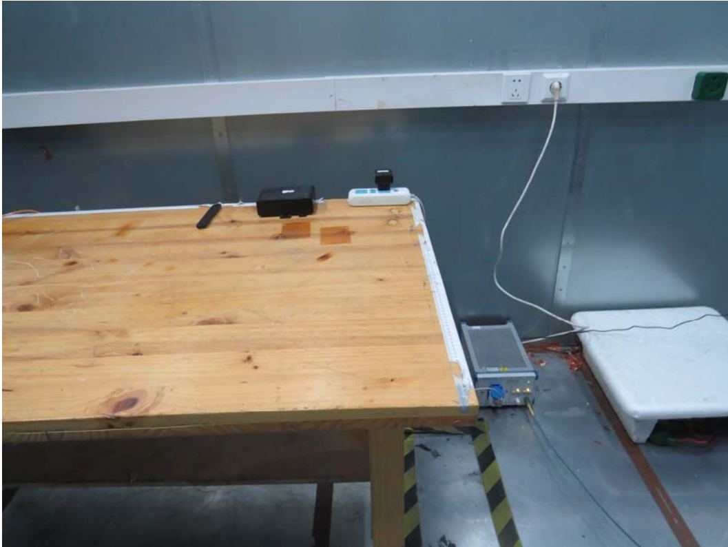
Picture 3 Conducted Emission Test Setup
