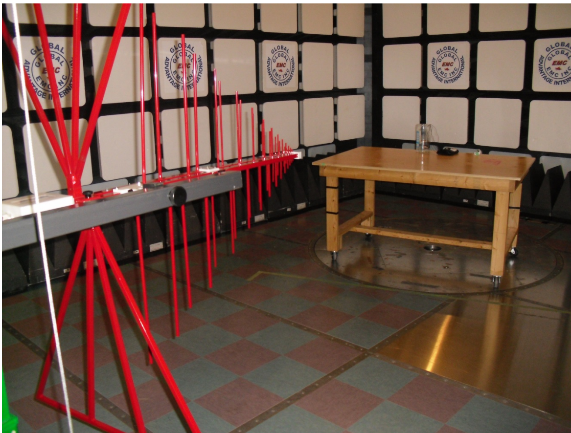
Radiated Emission Test Set-up _ Photo 2
