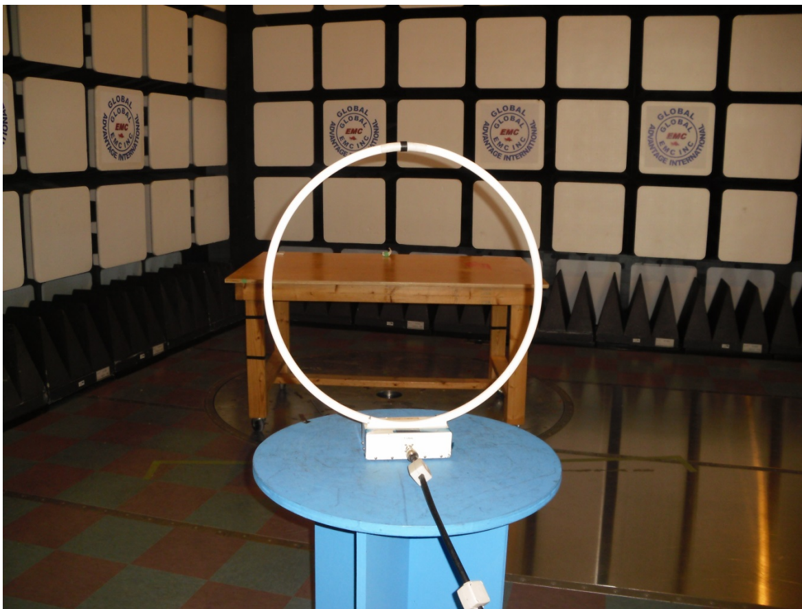
Radiated Emission Test Set-up _ Photo 1
