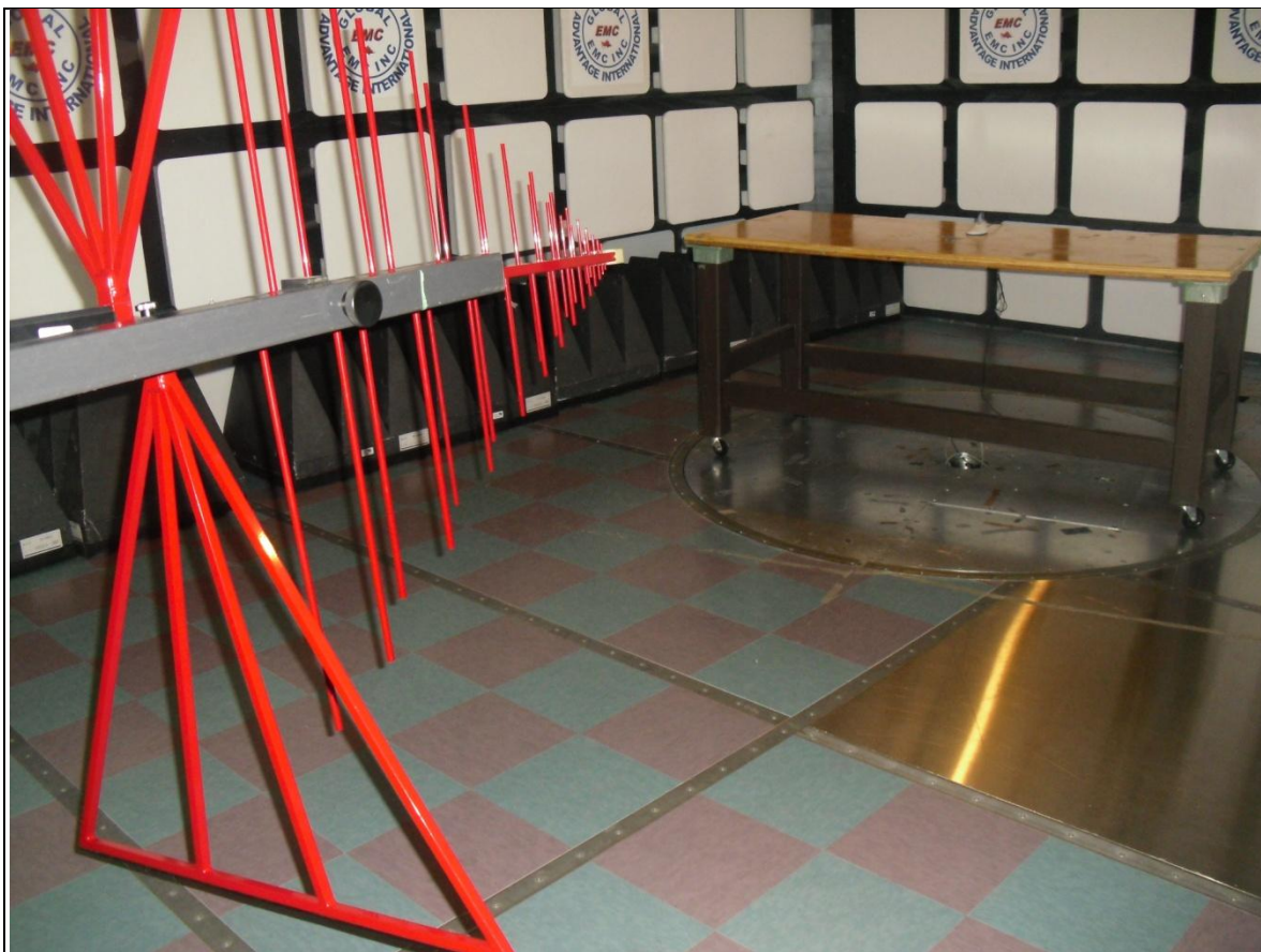
Radiated Emissions Test Set up _ Photo 1
