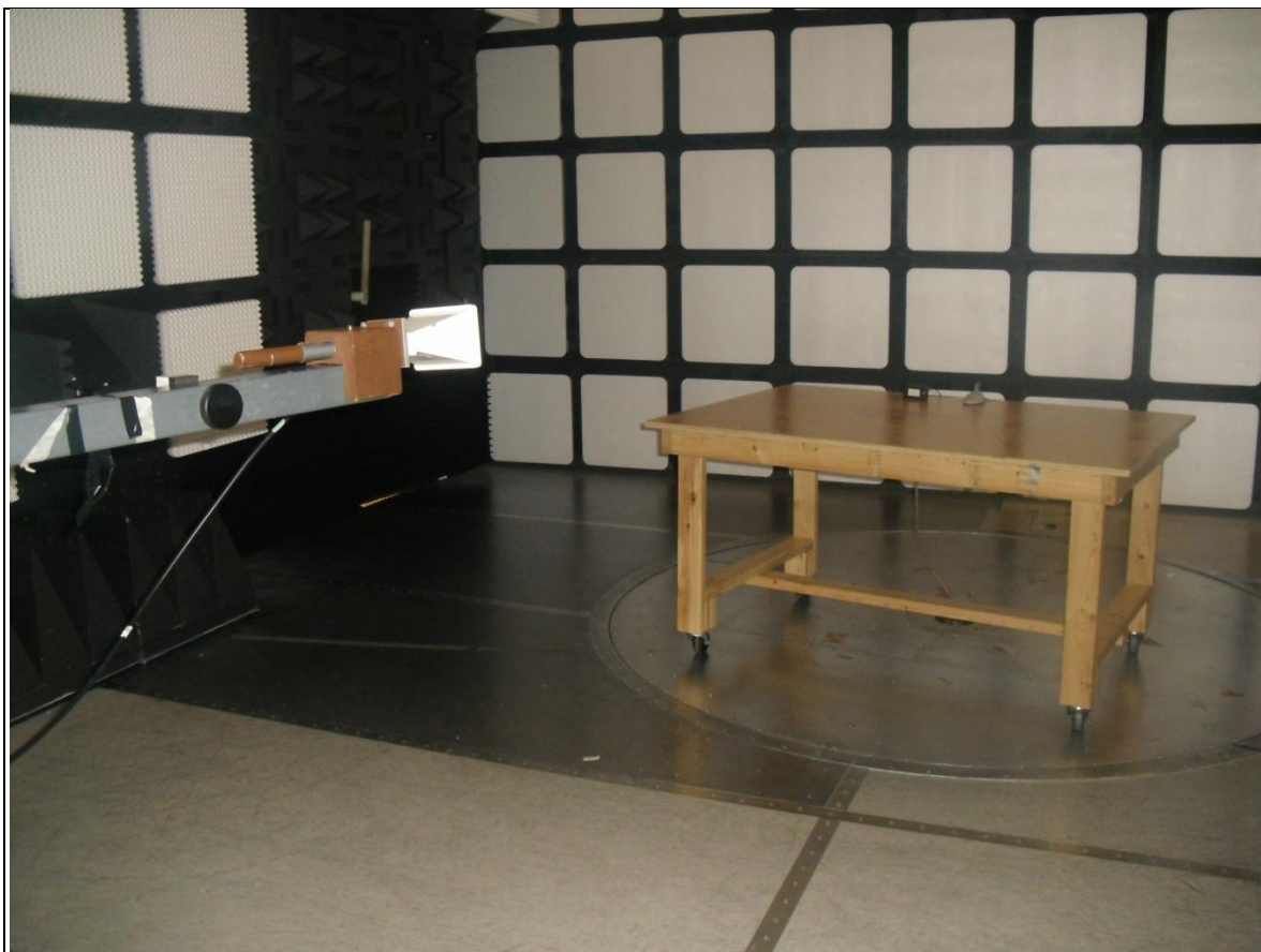
Radiated Emissions Test Set up _ Photo 2
