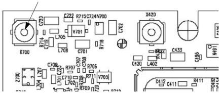
Figure 8: GPS antenna connector placement
