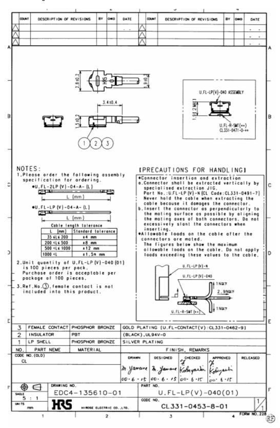
Figure 7: Specifications of U.FL-LP-(V)-040(01) plug
