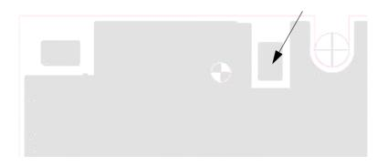
Figure 3: GSM antenna pad placement
