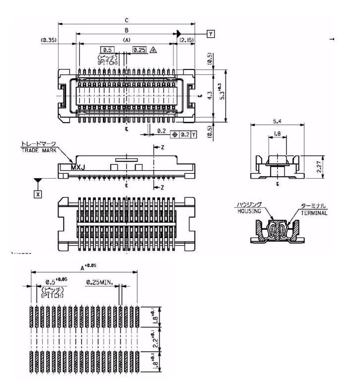
Figure 14: Molex board-to-board connector 52991-0808 on XT65/XT75
