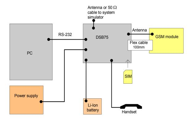
Figure 16: Reference equipment for Type Approval
