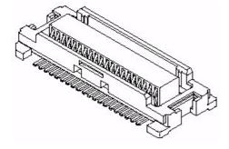
Type: 52991-0808 SlimStack Receptacle 80 pins, 0.50mm pitch, for stacking heights from 3.0 to 4.0mm, see Figure 14 for details.
