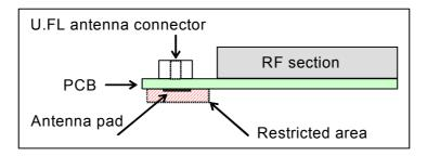
Figure 2: Figure 41: Restricted area around antenna pad
