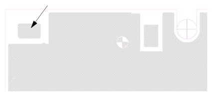
Figure 9: GPS antenna pad placement
