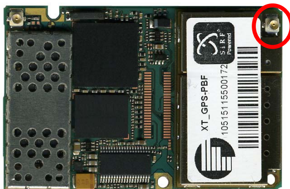
Figure 35: GPS antenna connector (U.FL-R-SMT connector)
