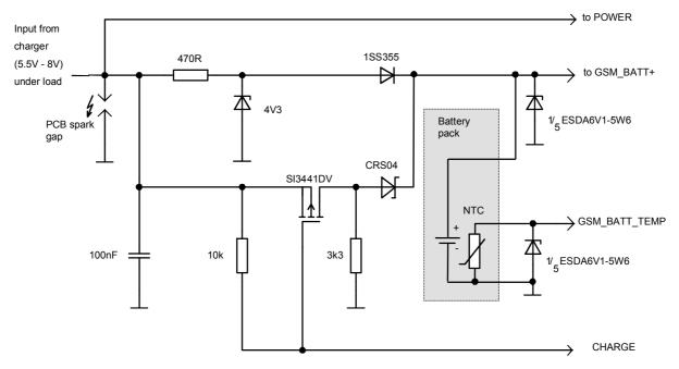
Figure 9: Schematic of approved charging transistor, trickle charging and ESD protection
