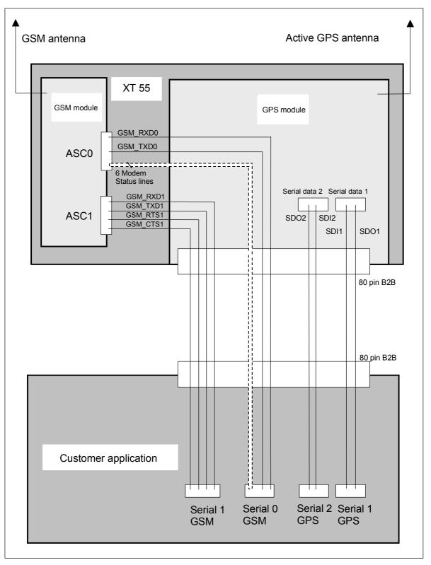
Figure 1: Block diagram of serial interface concept
