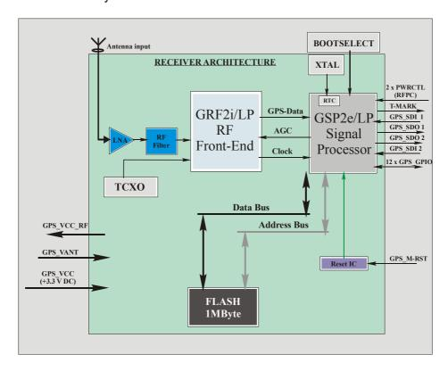
Figure 32: Receiver architecture of the GPS receiver
