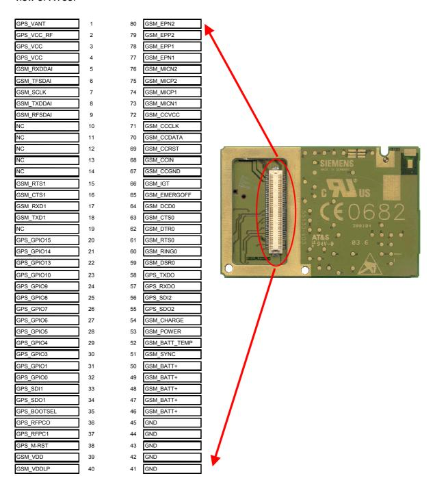
Figure 42: Pin assignment (top view on XT55)
