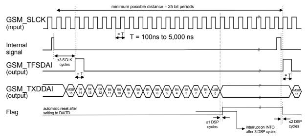
Figure 20: DAI timing on receive path
