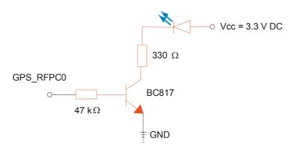
Figure 31: Example of LED circuit
