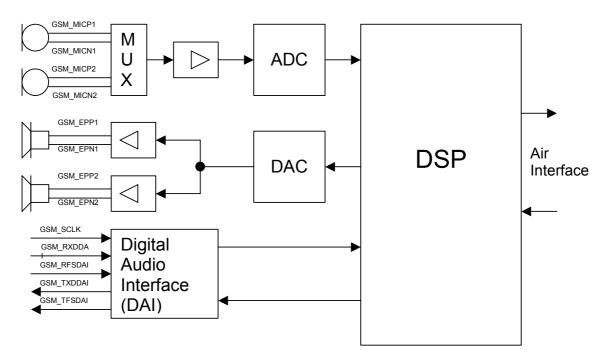
Figure 17: Audio block diagram
