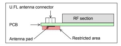
Figure 36: Restricted area around antenna pad
