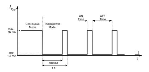
Figure 29: Example for current in Trickle Power mode
