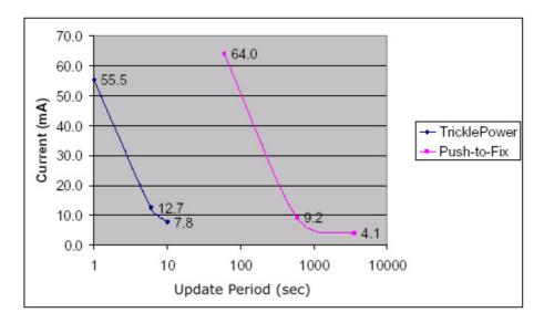
Figure 30: Current comparison between Trickle Power and Push-to Fix mode
