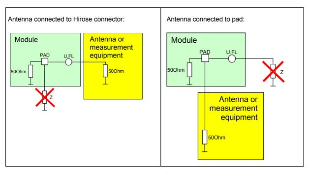
Figure 35: Never use antenna connector and antenna pad at the same time
