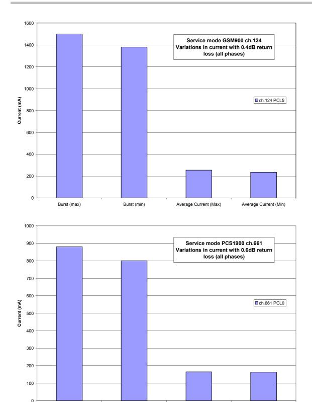
Test conditions:  $T_{amb}$ = 25°C,  $V_{GSM\_BATT+\ nom}$  = 4.1V measured at TP GSM\_BATT+ and GND, 1 TX slot Figure 49: Typical current consumption vs. return loss
