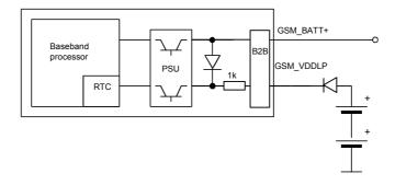
Figure 16: RTC supply from non-chargeable battery
