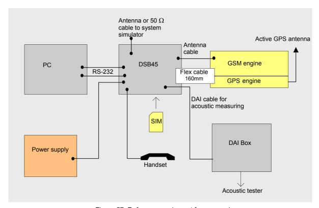
Figure 57: Reference equipment for approval
