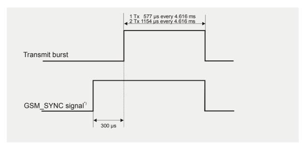
Figure 23: GSM\_SYNC signal during transmit burst
