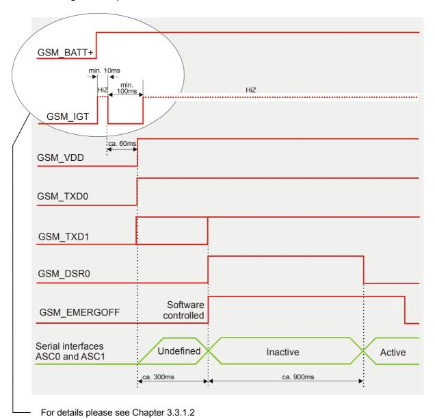
Figure 5: Power-on by ignition signal
