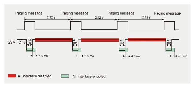
Figure 12: Timing of CTS signal (example for a 2.12 s paging cycle)
