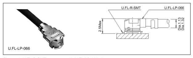
Figure 40: U.FL-R-SMT connector with U.FL-LP-066 plug
