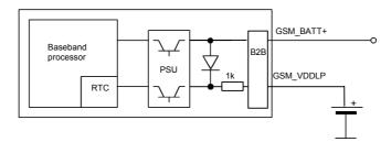
Figure 15: RTC supply from rechargeable battery
