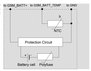
Figure 10: Battery pack circuit diagram
