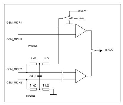
Figure 18: Schematic of microphone inputs
