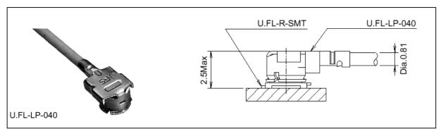
Figure 39: U.FL-R-SMT connector with U.FL-LP-040 plug
