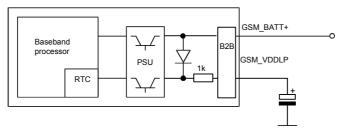
Figure 14: RTC supply from capacitor
