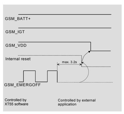
Figure 8: Deactivating GSM engine by GSM EMERGOFF signal
