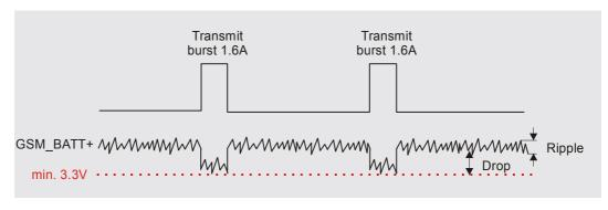
Figure 4: Power supply limits during transmit burst
