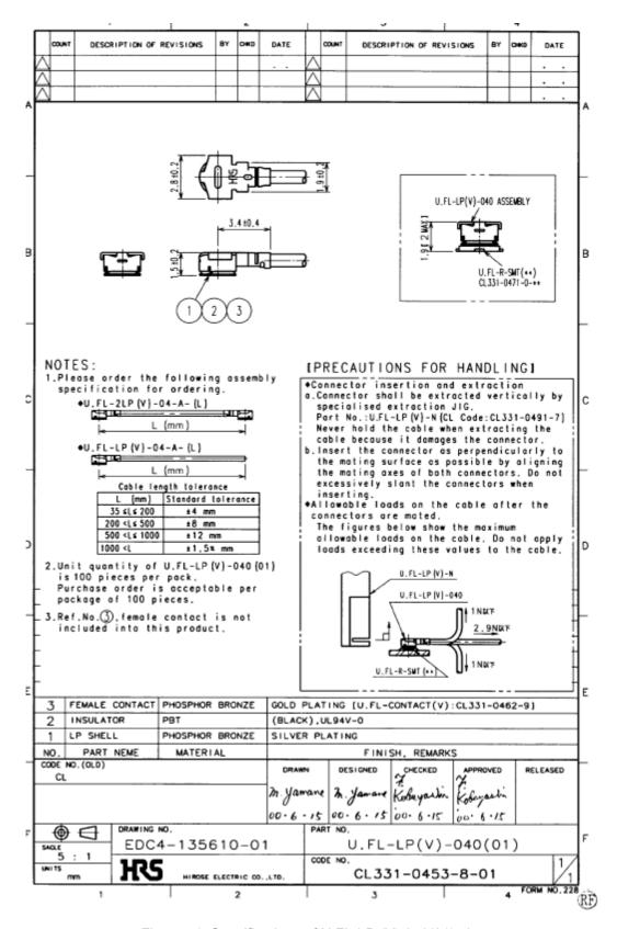
Figure 41: Specifications of U.FL-LP-(V)-040(01) plug
