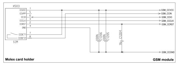
Figure 21: SIM card holder of DSB45 Support Box
