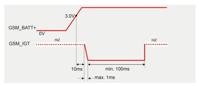
Figure 7: Timing of power-on process if GSM\_VDDLP is fed from external source
