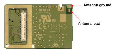
Figure 34: Antenna pad and GND plane
