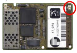
Figure 37: GPS antenna connector (U.FL-R-SMT connector)
