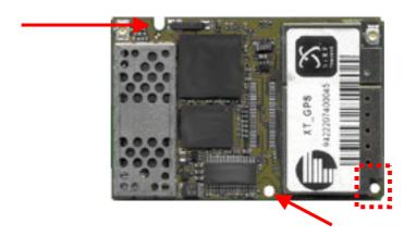
Figure 54: Mounting holes on XT55
