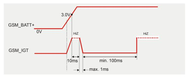
Figure 6: Timing of power-on process if GSM VDDLP is not used
