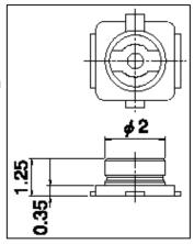
Figure 38: Mechanical dimensions of U.FL-R-SMT connector
