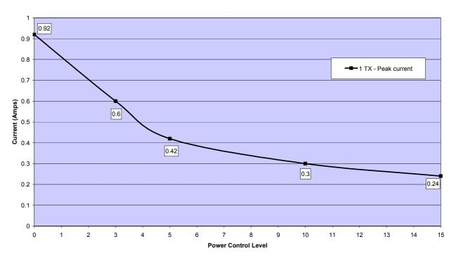
Test conditions: T<sub>amb</sub>= 25°C, V<sub>GSM\_BATT+ nom</sub> = 4.1V
