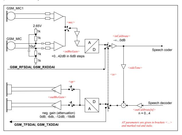
Figure 50: AT audio programming model
