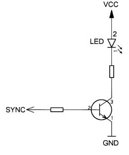
Figure 24: LED Circuit (Example)
