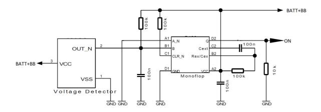
Figure 38: Automatic switch ON circuit sample
