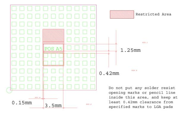
Figure 56: Dimensions of area for possible markings TX62-W (bottom view)
