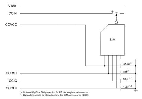
Figure 14: External UICC/SIM/USIM card holder circuit
