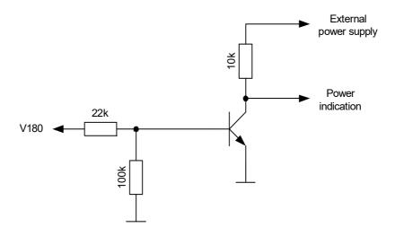
Figure 23: Power indication circuit
