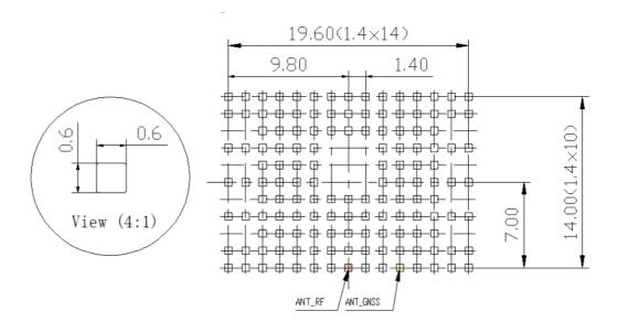
**Figure 64:** Recommended design for 110μm thick stencil for TX82-W, TX82-W-B, TX62-W-B and TX62-W-C (top view)
