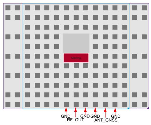
Figure 26: Antenna pads (top view)
