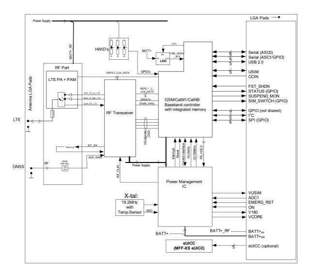
Figure 5: TX62-W-B block diagram
