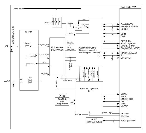
Figure 4: TX62-W block diagram
