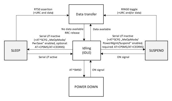
Figure 41: Low power modes with state transitions
