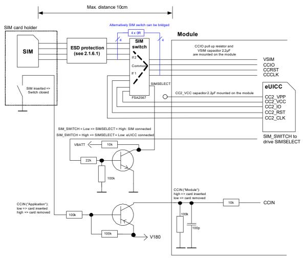
Figure 16: eUICC interface with switch for external SIM
