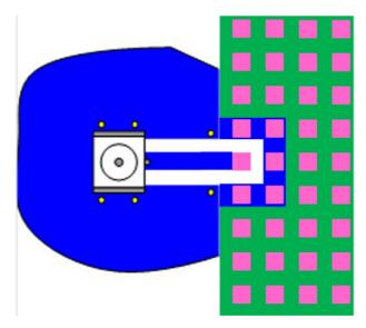
Figure 32: Routing to application's RF connector - top view
