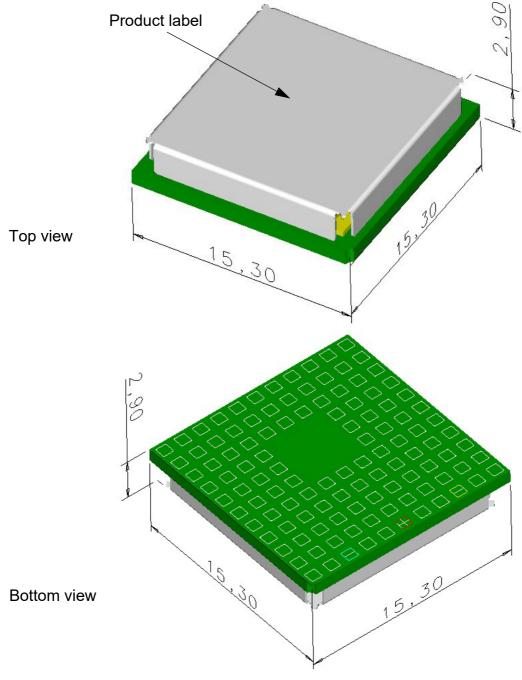
Figure 54: TX62-W- top and bottom view
