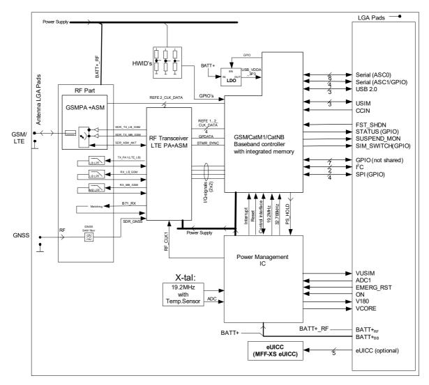
Figure 2: TX82-W block diagram
