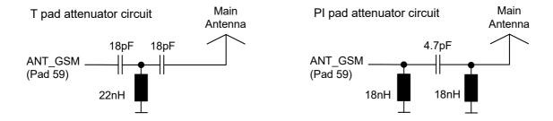
Figure 52: ESD protection for RF antenna interface
