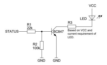
Figure 22: Status signaling with LED driver
