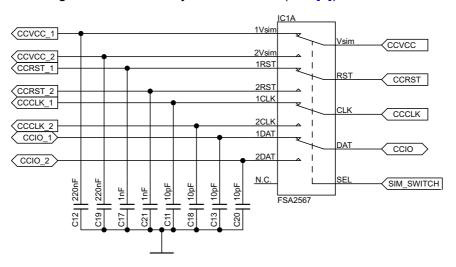
Figure 25: SIM switch circuit
