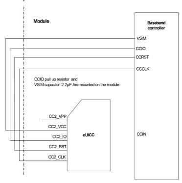
Figure 17: eUICC interface without SIM switch
