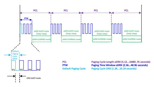
Figure 48: eDRX based paging and power saving in LTE Cat M1 and Cat NB1/2 networks
