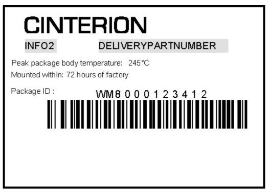
Figure 69: Barcode label on tape reel - layout
