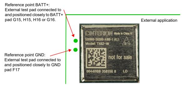
Figure 51: Position of reference points BATT+ and GND
