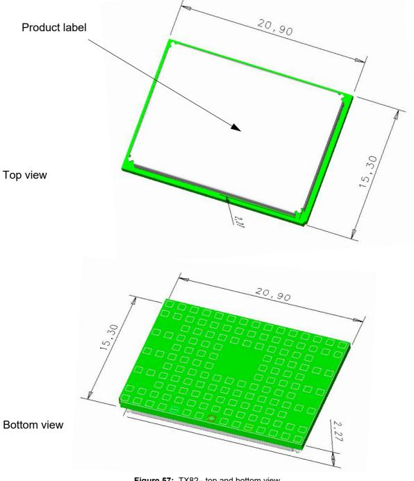
Figure 57: TX82- top and bottom view
