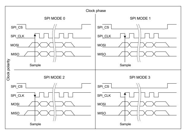
Figure 21: Characteristics of SPI modes
