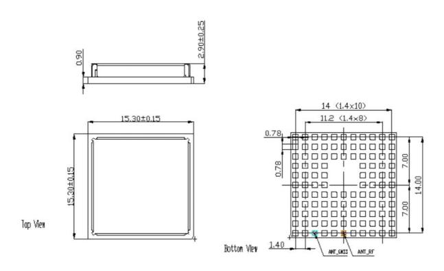
Figure 55: Dimensions of TX62-W (all dimensions in mm)
