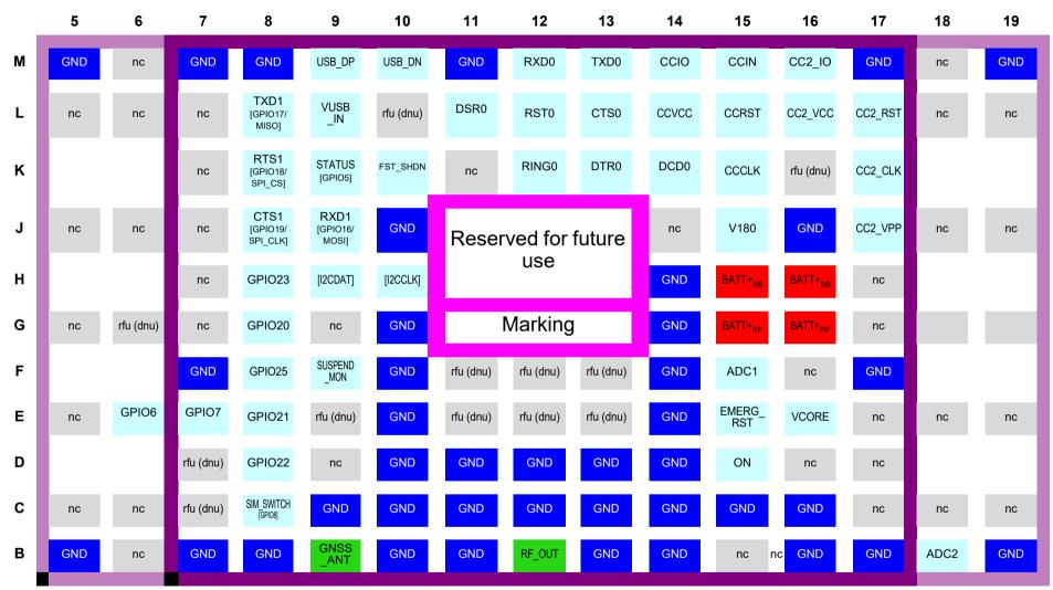
Figure 8: TX62/TX82 bottom view: Pad assignments
