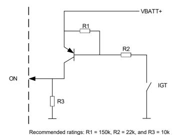
Figure 36: Sample ON circuit
