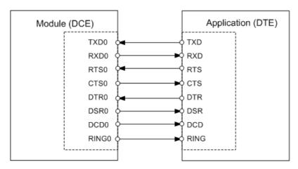
Figure 10: Serial interface ASC0
