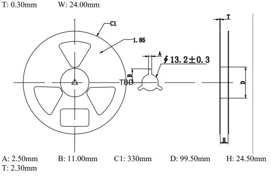
Figure 66: Carrier tape (TX62-W only)
