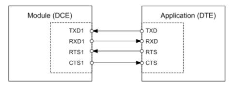
Figure 12: Serial interface ASC1
