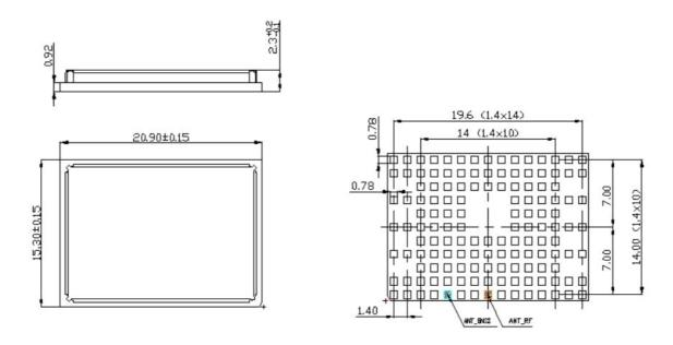
Figure 58: Dimensions of TX82-W and TX62-W-B (all dimensions in mm)
