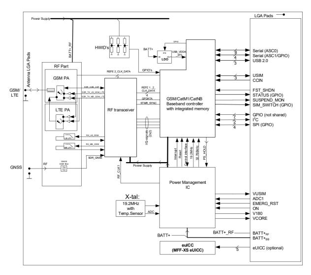
Figure 3: TX82-W-B block diagram
