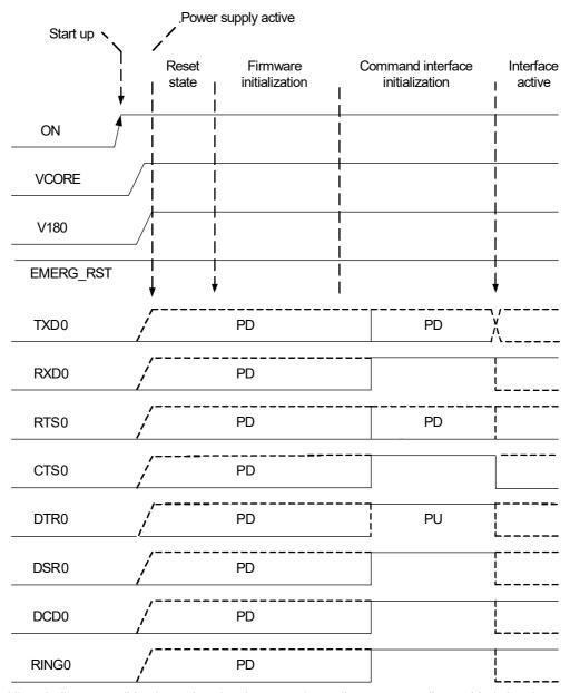
Dotted lines indicate possible alternative signal states - depending on externally provided signal states. For pull-up and pull-down values see Table 18.
