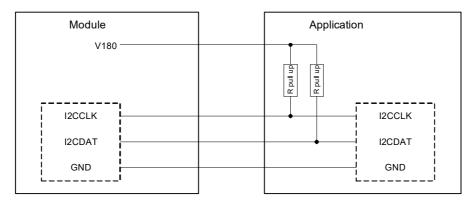
Figure 20: I<sup>2</sup>C interface connected to V180
