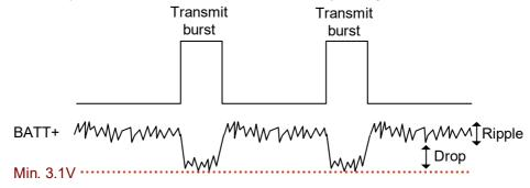
Figure 50: Power supply limits during transmit burst
