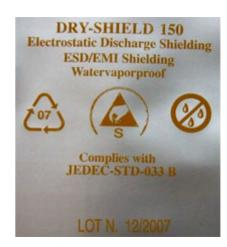
Figure 70: Moisture barrier bag (MBB) with imprint
