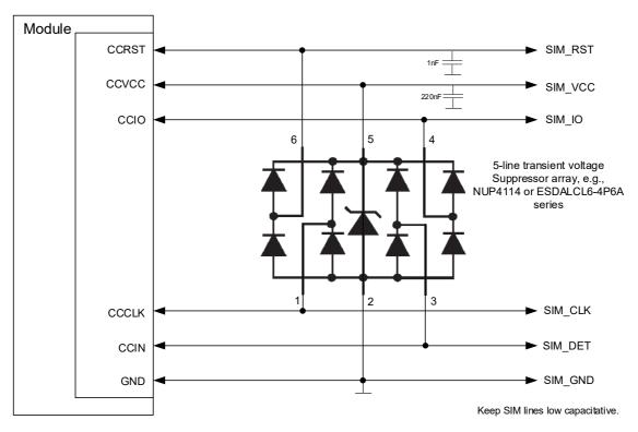
Figure 15: SIM interface - enhanced ESD protection
