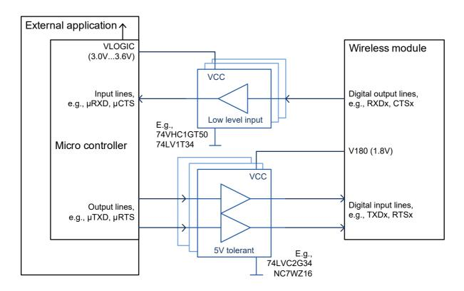
Figure 35: Sample level conversion circuit
