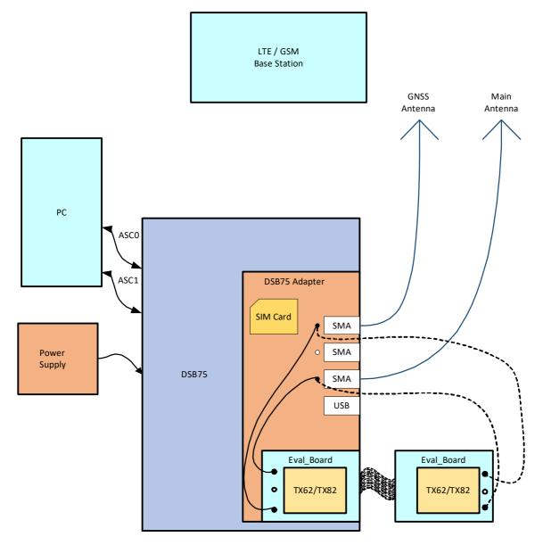
Figure 78: Reference equipment for type approval
