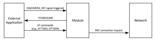
Figure 44: Handshake for module wake up via ON signal
