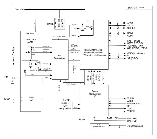
Figure 6: TX62-W-C block diagram
