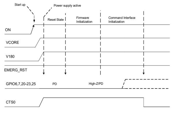
Figure 19: GPIO start up behavior
