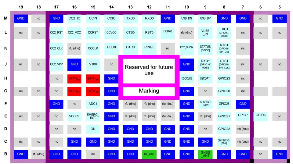
Figure 7: TX62/TX82 top view: Pad assignments
