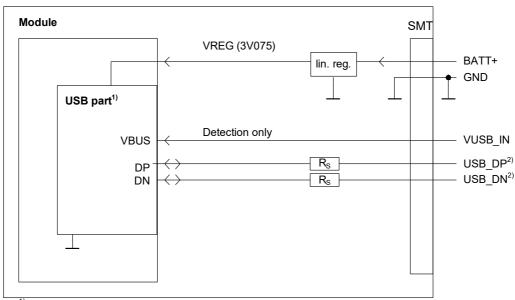
$<sup>^{1)}</sup>$  All serial (including  $R_{\rm S}$ ) and pull-up resistors for data lines are implemented.
