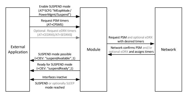
Figure 43: Handshake for entering the module's SUSPEND mode
