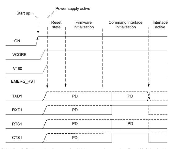
Dotted lines indicate possible alternative signal states - depending on externally provided signal states. \*) For pull-down values see Table 18.
