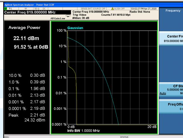
3.75KHz Sub-carrier spacing, QPSK
