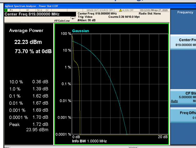
15KHz Sub-carrier spacing, QPSK
