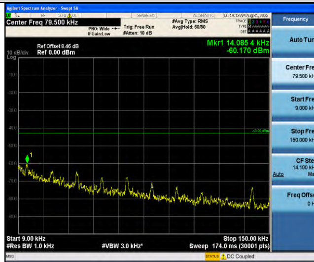
Band66-Stand-Alone-NaN-BPSK-132670-1 @ 11-15kHz-0.009-0.15-0.009~0.15MHz @ -60.17dBm--43-PASS
