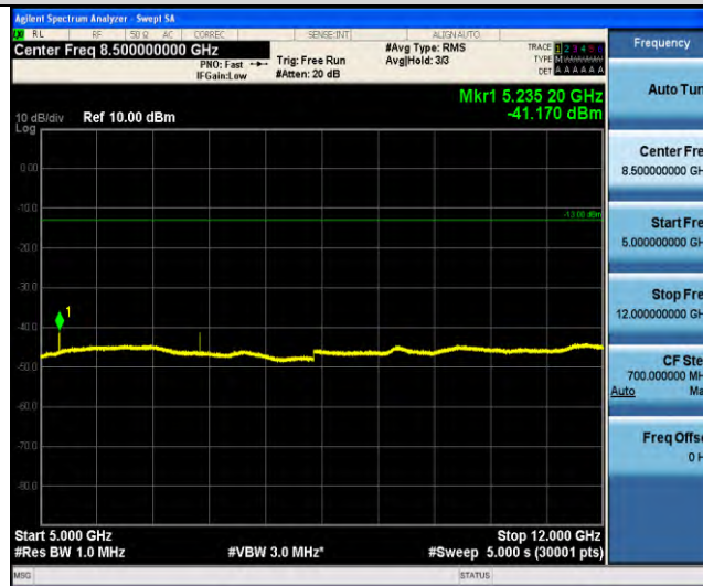
Band66-Stand-Alone-NaN-QPSK-132322-1 @47-3.75kHz-5000-12000-5000~12000MHz @-41.17dBm--13-PASS
