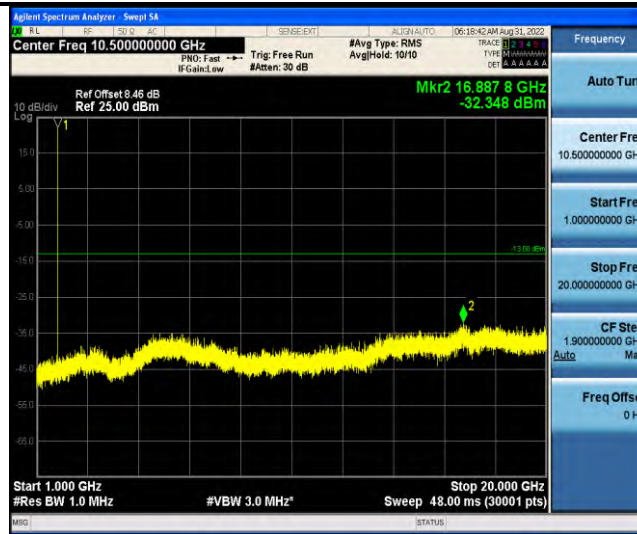
Band66-Stand-Alone-NaN-BPSK-132670-1 @ 0-15kHz-1000-20000-1000~20000MHz @ -32.35dBm--13-PASS
