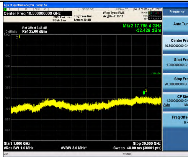
Band66-Stand-Alone-NaN-BPSK-132670-1 @ 11-15kHz-1000-20000-1000~20000MHz @ -32.43dBm--13-PASS
