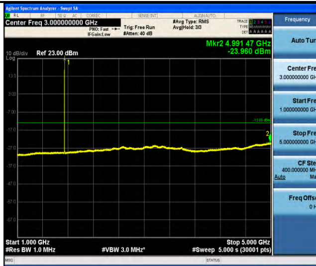
Band66-Stand-Alone-NaN-QPSK-132322-1 @0-3.75kHz-1000-5000-1000~5000MHz@ -23.96dBm--13-PASS
