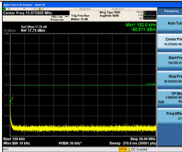
Band66-Stand-Alone-NaN-BPSK-132322-1 @ 11-15kHz-0.15-30-0.15~30MHz @ -50.51dBm--33-PASS
