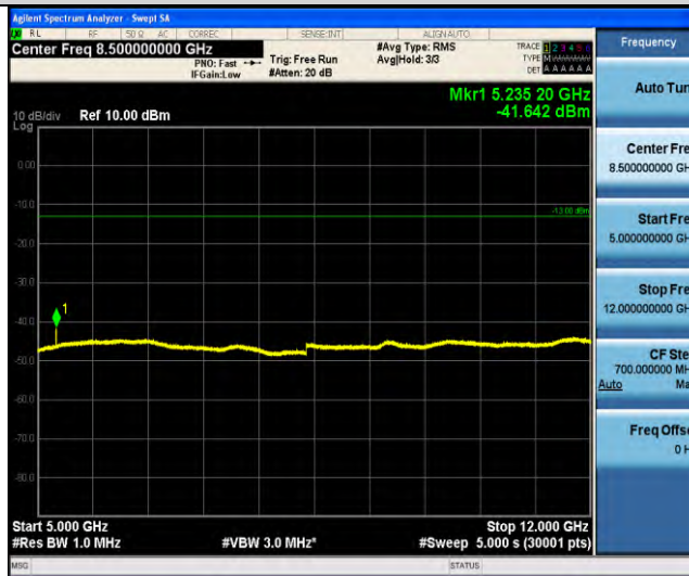
Band66-Stand-Alone-NaN-QPSK-132322-1 @0-3.75kHz-5000-12000-5000~12000MHz@ -41.64dBm--13-PASS
