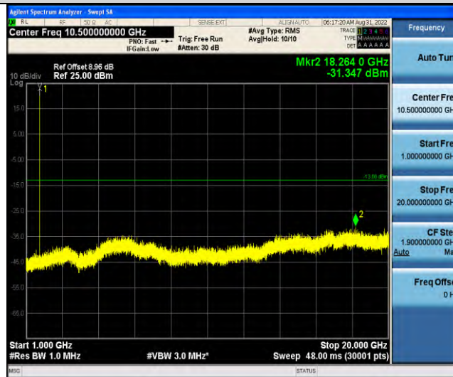
Band66-Stand-Alone-NaN-BPSK-131974-1 @ 11-15kHz-1000-20000-1000~20000MHz @ -31.35dBm--13-PASS
