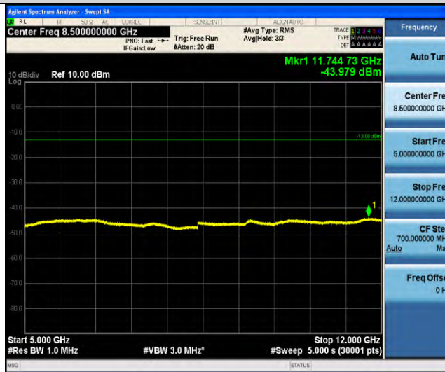
Band66-Stand-Alone-NaN-BPSK-132322-1 @ 11-15kHz-5000-12000-5000~12000MHz @ -43.98dBm--13-PASS
