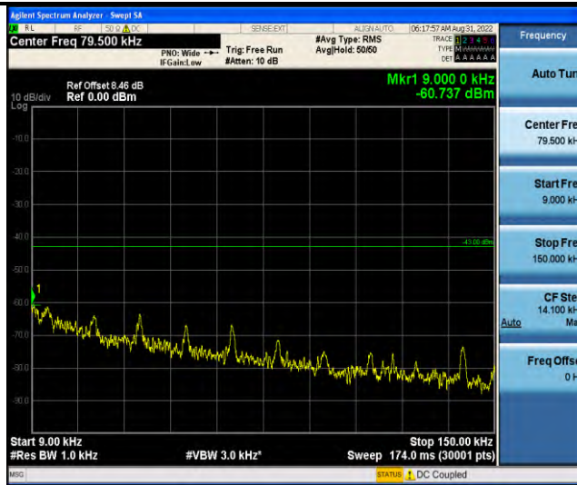
Band66-Stand-Alone-NaN-BPSK-132670-1 @ 0-15kHz-0.009-0.15-0.009~0.15MHz @ -60.74dBm--43-PASS
