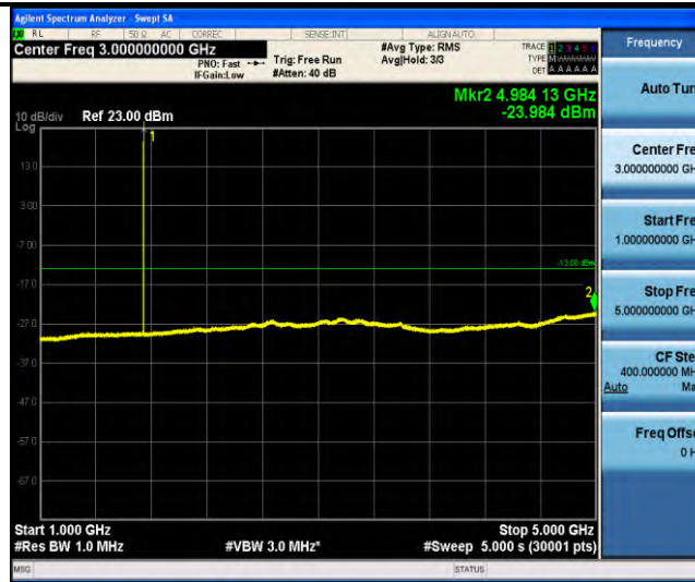
Band66-Stand-Alone-NaN-QPSK-132322-1 @47-3.75kHz-1000-5000-1000~5000MHz @-23.98dBm--13-PASS
