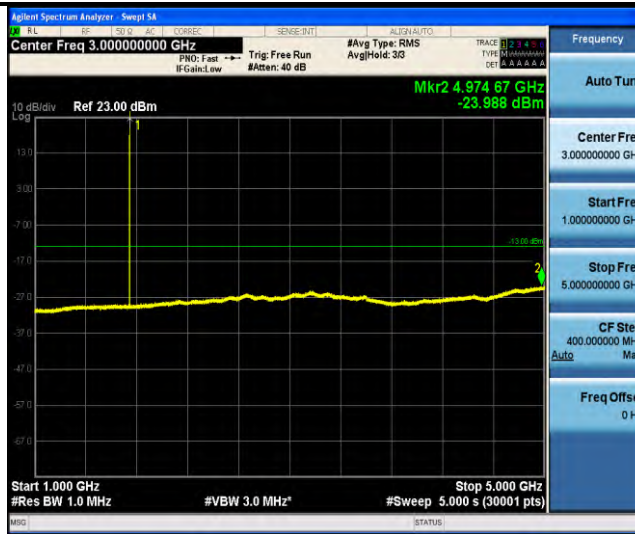
Band66-Stand-Alone-NaN-BPSK-132322-1 @ 11-15kHz-1000-5000-1000~5000MHz @ -23.99dBm--13-PASS
