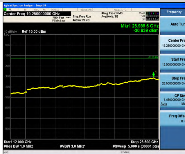
Band66-Stand-Alone-NaN-QPSK-132322-1 @47-3.75kHz-12000-26500-12000~26500MHz @-30.94dBm--13-PASS
