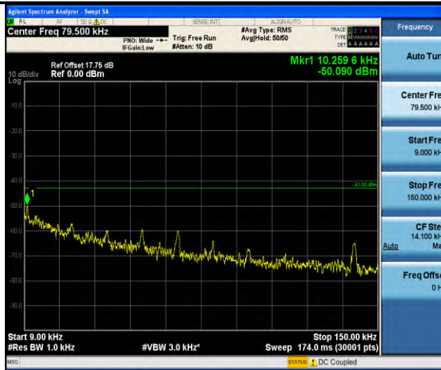
Band66-Stand-Alone-NaN-BPSK-132322-1 @ 11-15kHz-0.009-0.15-0.009~0.15MHz @ -50.09dBm--43-PASS
