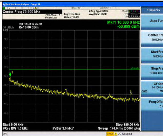
Band66-Stand-Alone-Na-N-QPSK-132322-1 @ 0-3.75kHz-0.009-0.15-0.009~0.15MHz @ -50.9dBm--43-PASS
