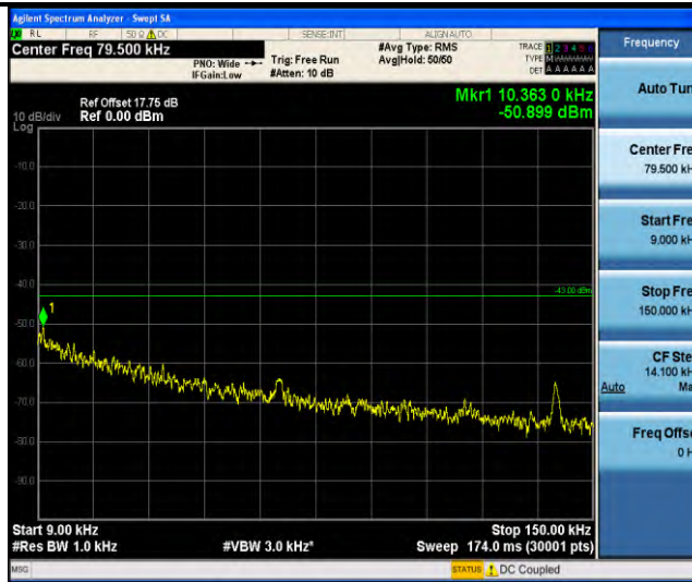
Band66-Stand-Alone-NaN-QPSK-132322-1 @ 0-3.75kHz-0.009-0.15-0.009-0.15MHz @ -50.9dBm--43-PASS
