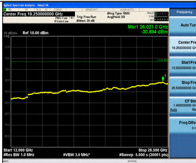
Band66-Stand-Alone-NaN-BPSK-132322-1 @ 11-15kHz-12000-26500-12000~26500MHz @ -30.89dBm--13-PASS
