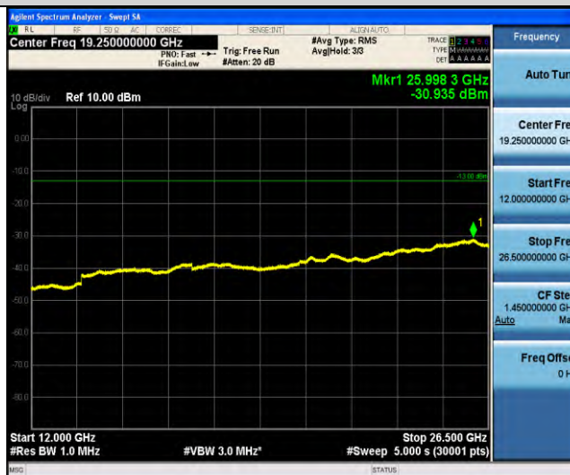
Band66-Stand-Alone-NaN-QPSK-132322-1 @0-3.75kHz-12000-26500-12000~26500MHz@ -30.94dBm--13-PASS
