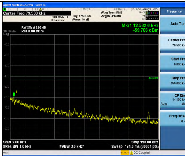
Band66-Stand-Alone-NaN-QPSK-131974-1 @ 0-3.75kHz-0.009-0.15-0.009~0.15MHz @ -59.79dBm--43-PASS
