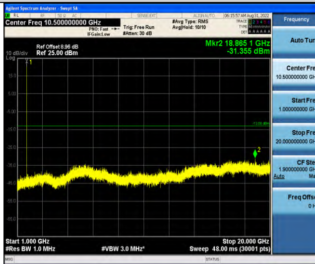
Band66-Stand-Alone-NaN-BPSK-131974-1 @0-15kHz-1000-20000-1000~20000MHz @ -31.36dBm--13-PASS
