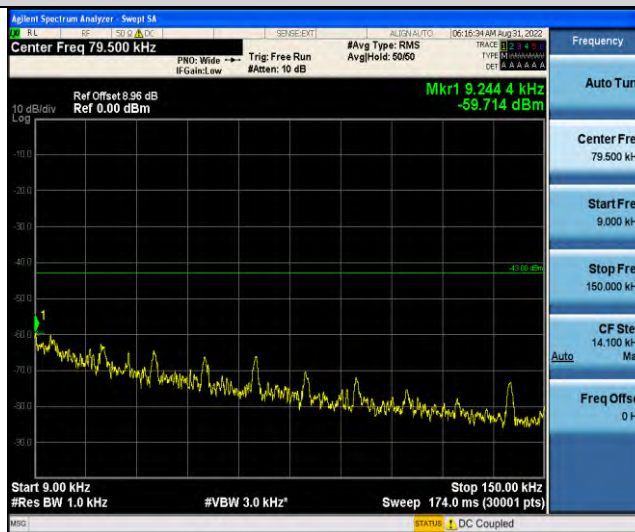
Band66-Stand-Alone-NaN-BPSK-131974-1 @11-15kHz-0.009-0.15-0.009~0.15MHz @ -59.71dBm--43-PASS
