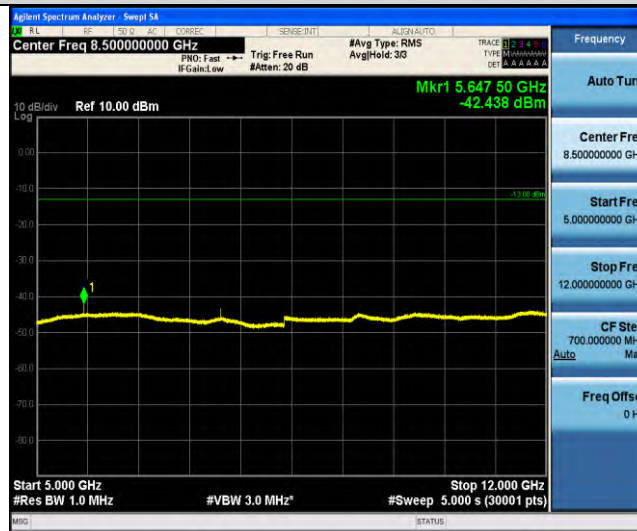
Band25-Stand-Alone-NaN-BPSK-26365-1 @ 0-15kHz-5000-12000-5000~12000MHz @ -42.44dBm--13-PASS
