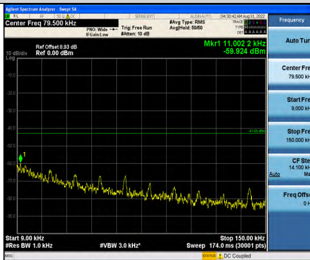
Band25-Stand-Alone-NaN-QPSK-26042-12 @ 0-15kHz-0.009-0.15-0.009~0.15MHz @ -59.92dBm--43-PASS
