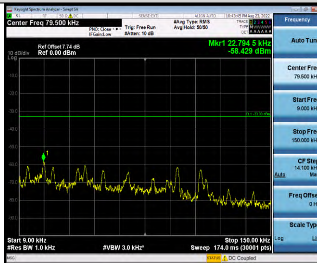
Band19-Stand-Alone-NaN-QPSK-24002-12 @ 0-15kHz-0.009-0.15-0.009~0.15MHz @ -58.43dBm--33-PASS
