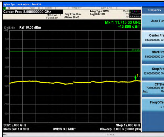
Band19-Stand-Alone-NaN-QPSK-24075-1 @ 47-3.75kHz-5000-12000-5000~12000MHz @ -43.9dBm--13-PASS
