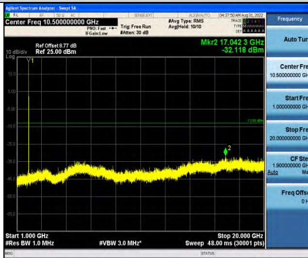
Band25-Stand-Alone-NaN-BPSK-26688-1 @ 11-15kHz-1000-20000-1000~20000MHz @ -32.12dBm--13-PASS
