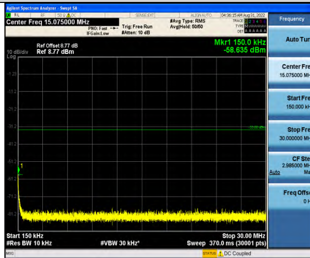
Band25-Stand-Alone-Na-N-BPSK-26688-1 @ 0-15kHz-0.15-30-0.15~30MHz @ -58.64dBm--33-PASS
