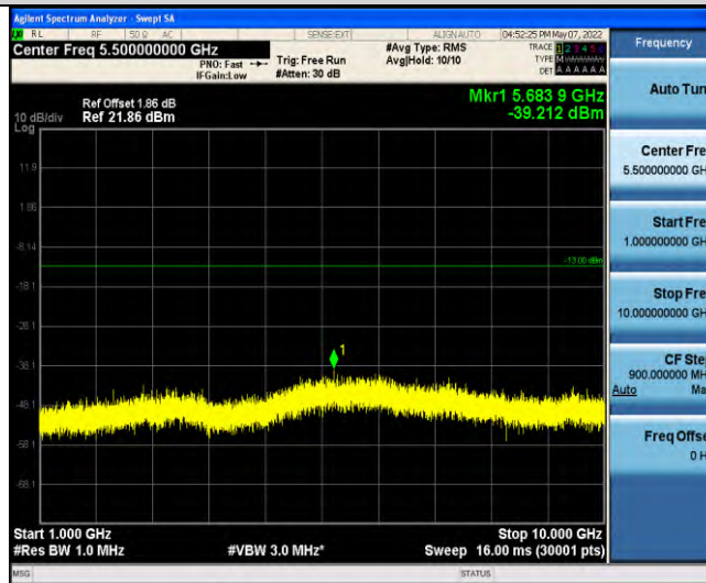
Band17-Stand-Alone-Na-N-QPSK-23790-1 @0-3.75kHz-1000-10000-1000~10000MHz @ -39.21dBm--13-PASS
