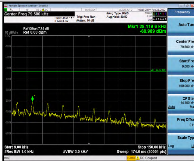
Band18-Stand-Alone-NaN-QPSK-23852-12 @ 0-15kHz-0.009-0.15-0.009~0.15MHz @ -60.99dBm--33-PASS
