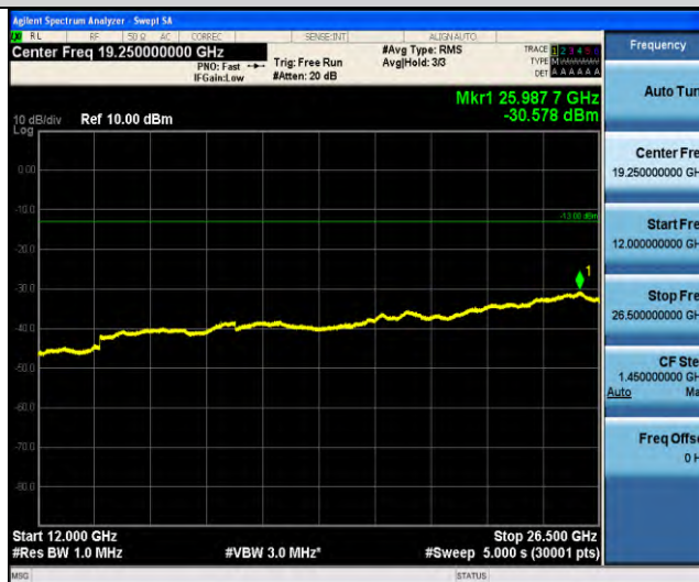
Band18-Stand-Alone-NaN-QPSK-23925-1 @47-3.75kHz-12000-26500-12000~26500MHz@ -30.58dBm--13-PASS
