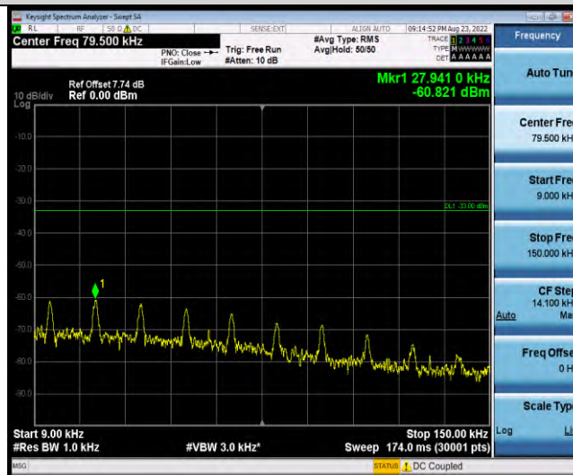
Band18-Stand-Alone-NaN-BPSK-23852-1 @ 11-15kHz-0.009-0.15-0.009~0.15MHz @ -60.82dBm--33-PASS
