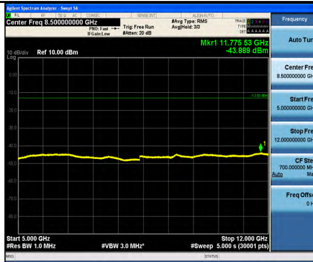
Band18-Stand-Alone-NaN-QPSK-23925-1 @0-3.75kHz-5000-12000-5000~12000MHz @-43.89dBm--13-PASS
