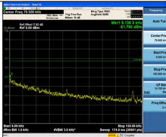
Band18-Stand-Alone-NaN-QPSK-23925-1 @0-3.75kHz-0.009-0.15-0.009~0.15MHz@ -51.79dBm--33-PASS
