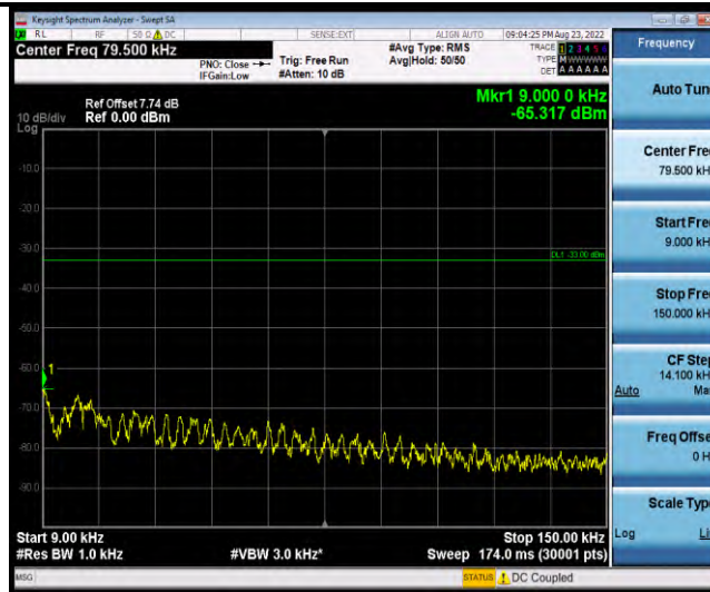
Band18-Stand-Alone-Na-N-QPSK-23852-1 @ 0-3.75kHz-0.009-0.15-0.009~0.15MHz @ -65.32dBm--33-PASS
