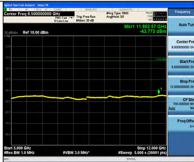
Band18-Stand-Alone-NaN-BPSK-23925-1 @ 11-15kHz-5000-12000-5000~12000MHz@ -43.77dBm--13-PASS
