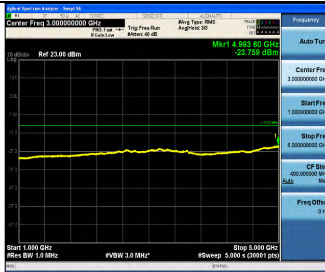
Band18-Stand-Alone-NaN-BPSK-23925-1 @ 11-15kHz-1000-5000-1000~5000MHz@ -23.76dBm--13-PASS
