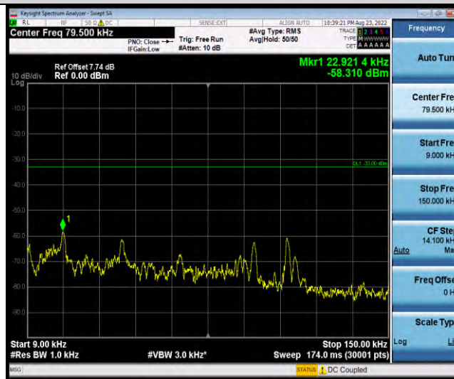
Band19-Stand-Alone-NaN-QPSK-24002-1 @ 47-3.75kHz-0.009-0.15-0.009~0.15MHz @ -58.31dBm--33-PASS
