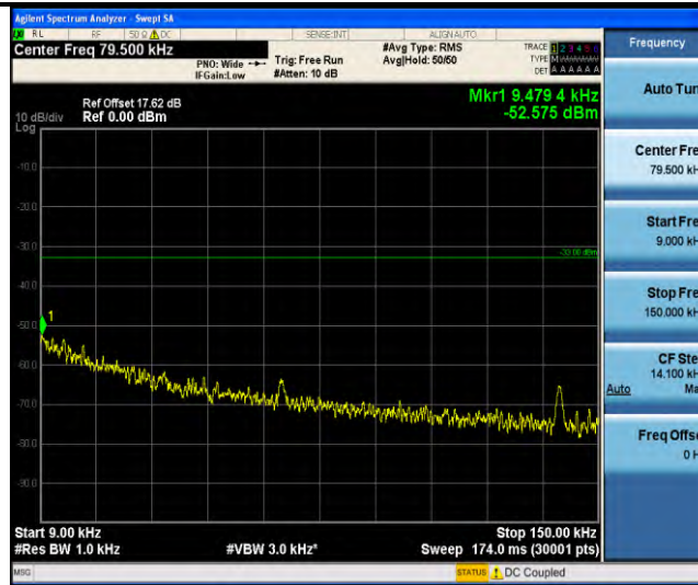
Band18-Stand-Alone-NaN-QPSK-23925-1 @ 47-3.75kHz-0.009-0.15-0.009~0.15MHz@ -52.58dBm--33-PASS
