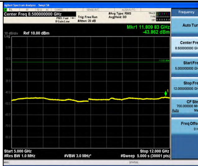
Band18-Stand-Alone-NaN-QPSK-23925-1 @47-3.75kHz-5000-12000-5000~12000MHz@ -43.86dBm--13-PASS
