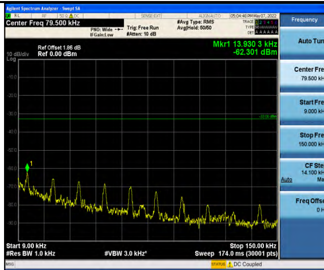
Band17-Stand-Alone-NaN-BPSK-23790-1 @ 11-15kHz-0.009-0.15-0.009~0.15MHz @ -62.3dBm--33-PASS
