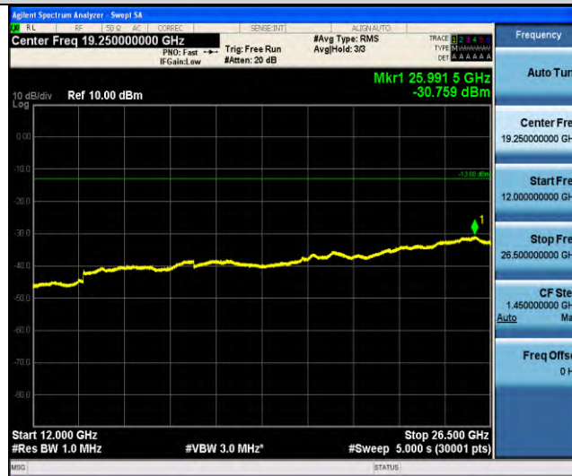
Band18-Stand-Alone-NaN-QPSK-23925-1 @0-3.75kHz-12000-26500-12000~26500MHz @-30.76dBm--13-PASS
