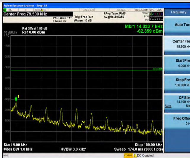
Band17-Stand-Alone-Na-N-BPSK-23790-1 @ 0-15kHz-0.009-0.15-0.009~0.15MHz @ -62.36dBm--33-PASS
