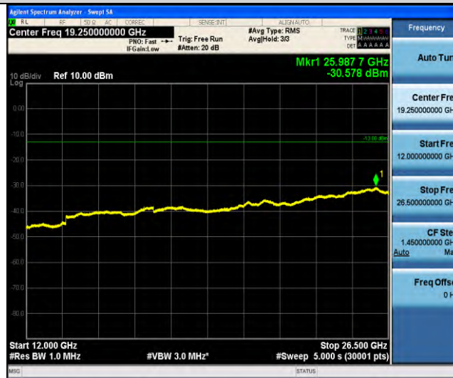
Band18-Stand-Alone-NaN-QPSK-23925-1 @47-3.75kHz-12000-26500-12000~26500MHz@ -30.58dBm--13-PASS
