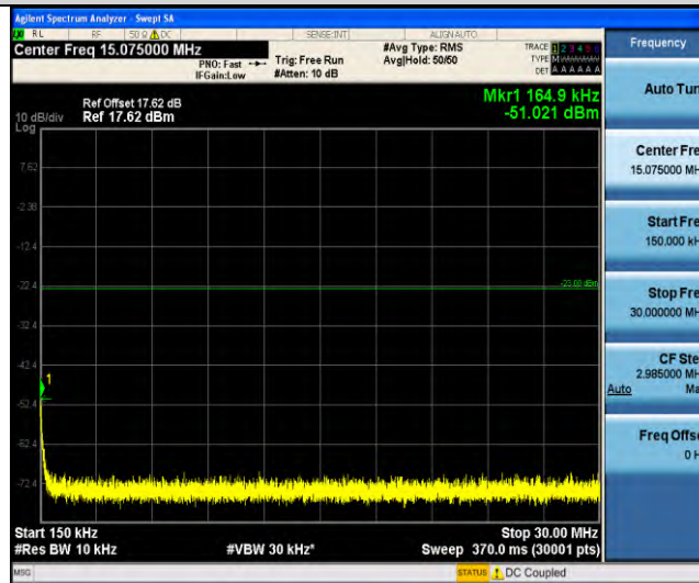
Band18-Stand-Alone-NaN-QPSK-23925-1 @ 47-3.75kHz-0.15-30-0.15~30MHz@ -51.02dBm--23-PASS
