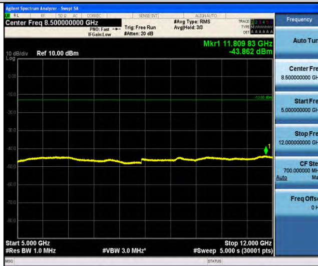
Band18-Stand-Alone-NaN-QPSK-23925-1 @47-3.75kHz-5000-12000-5000~12000MHz@ -43.86dBm--13-PASS
