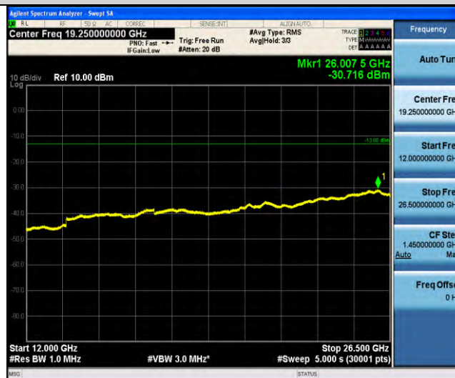
Band18-Stand-Alone-NaN-BPSK-23925-1 @ 11-15kHz-12000-26500-12000~26500MHz@ -30.72dBm--13-PASS
