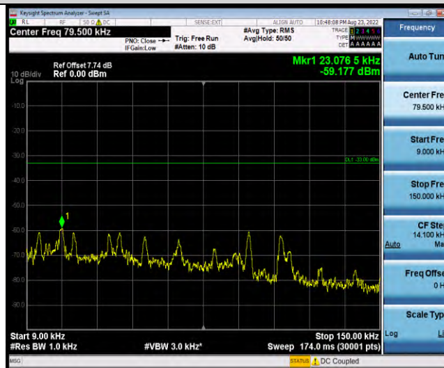
Band19-Stand-Alone-NaN-BPSK-24002-1 @ 11-15kHz-0.009-0.15-0.009~0.15MHz @ -59.18dBm--33-PASS
