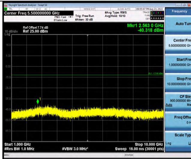
Band18-Stand-Alone-NaN-QPSK-23852-1 @0-3.75kHz-1000-10000-1000~1000MHz @-40.32dBm--13-PASS
