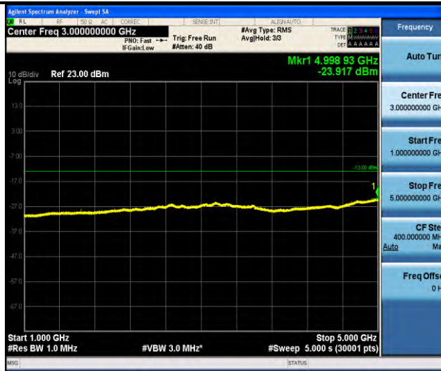
Band18-Stand-Alone-NaN-QPSK-23925-1 @47-3.75kHz-1000-5000-1000~5000MHz@ -23.92dBm--13-PASS
