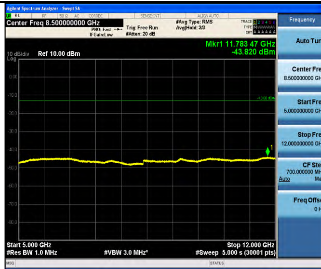
Band19-Stand-Alone-NaN-QPSK-24075-1 @0-3.75kHz-5000-12000-5000~12000MHz @-43.82dBm--13-PASS
