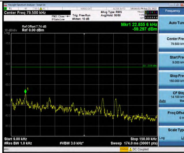
Band18-Stand-Alone-NaN-QPSK-23852-1 @ 47-3.75kHz-0.009-0.15-0.009~0.15MHz @ -59.3dBm--33-PASS
