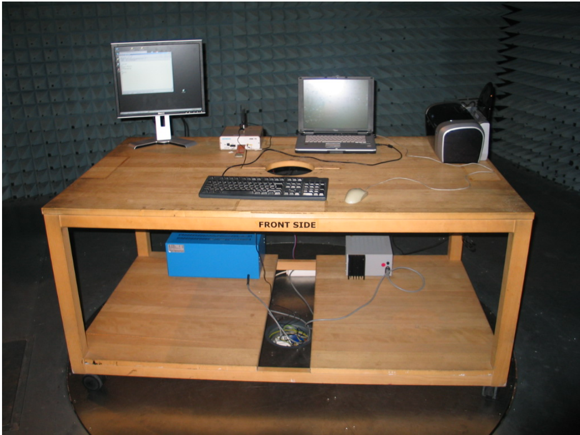
Photo 2: Test setup for radiated measurements
