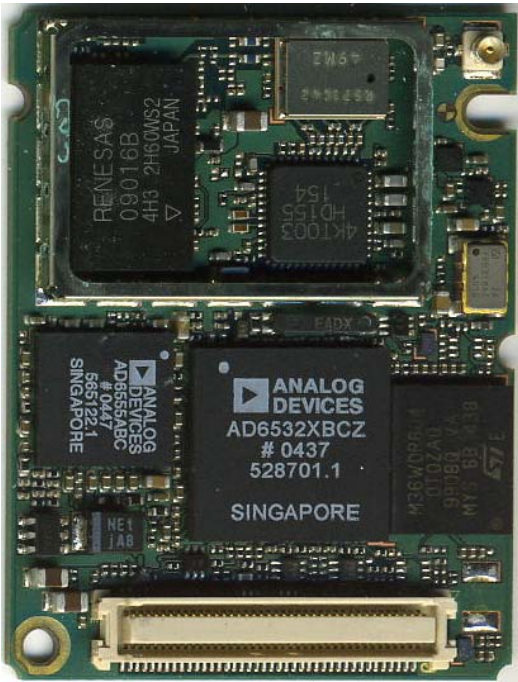
TC65: component side shielding opened
