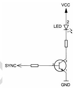
Figure 26: LED Circuit (Example)
