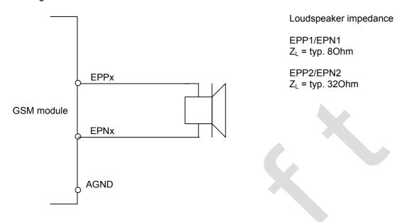
Figure 21: Differential loudspeaker configuration
