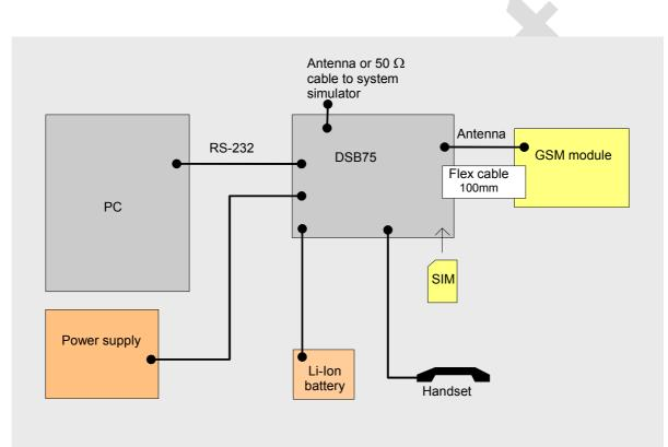
Figure 39: Reference equipment for Type Approval
