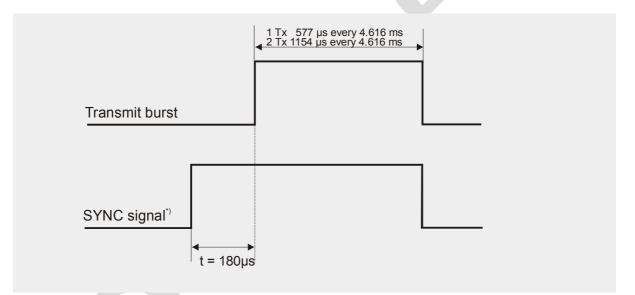
Figure 25: SYNC signal during transmit burst
