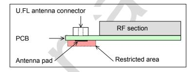
Figure 28: Restricted area around antenna pad
