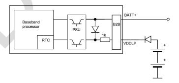
Figure 11: RTC supply from non-chargeable battery
