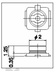
Figure 29: Mechanical dimensions of U.FL-R-SMT connector
