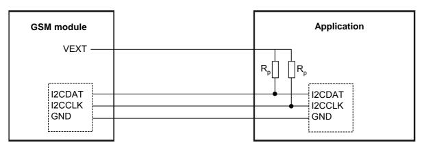
Figure 16: I<sup>2</sup>C interface connected to VEXT line of TC63
