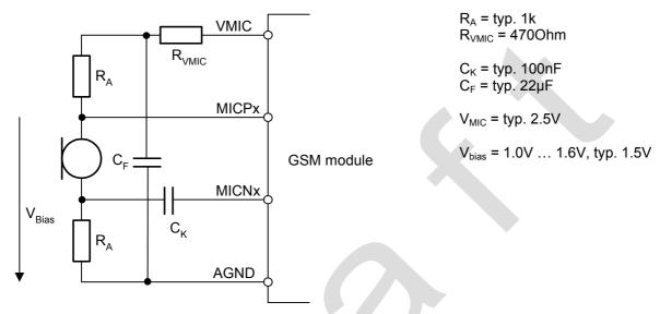
Figure 19: Differential microphone input
