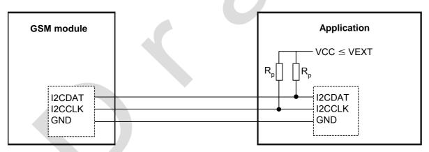
Figure 15: I<sup>2</sup>C interface connected to VCC of application
