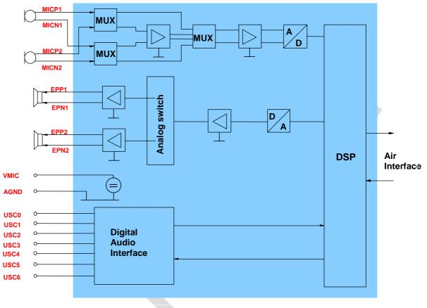
Figure 17: Audio block diagram
