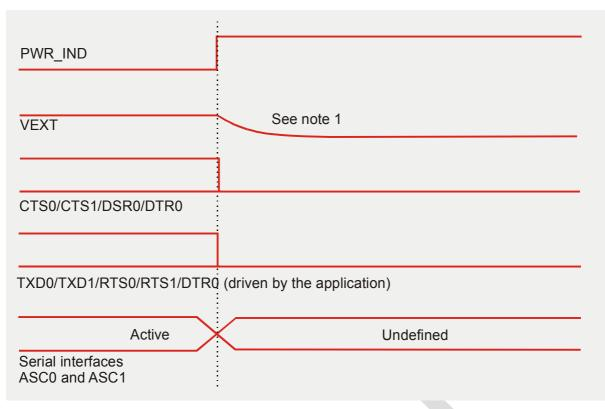
Figure 7: Signal states during turn-off procedure
