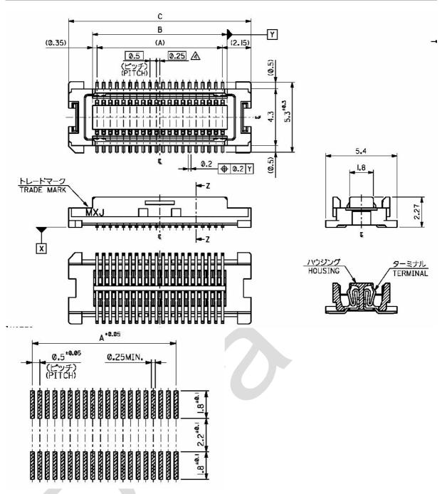
Figure 36: Molex board-to-board connector 52991-0808 on TC63
