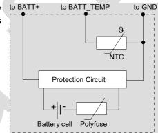
Figure 8: Battery pack circuit diagram
