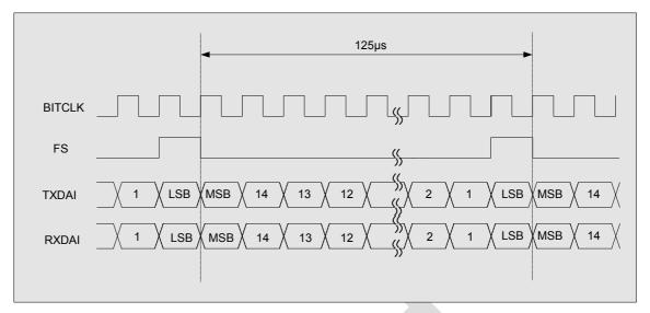
Figure 24: PCM timing
