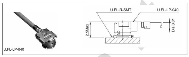
Figure 30: U.FL-R-SMT connector with U.FL-LP-040 plug
