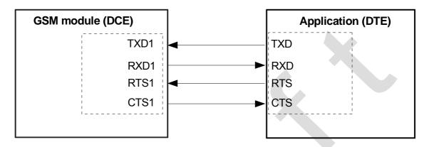
Figure 13: Serial interface ASC1
