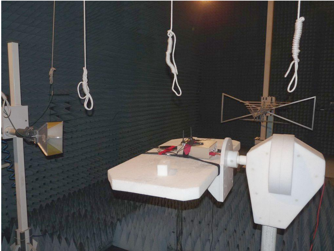
Photo 1: Test setup for radiated measurements (Enclosure, fully-anechoic chamber, 30 MHz – 10/20 GHz §22/24/90)
