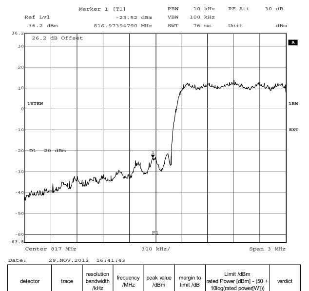
$$0.25\ \ \ W$$  Measured Level was corrected by 1 dB to correct measurement bandwidth to 12.5 kHz
